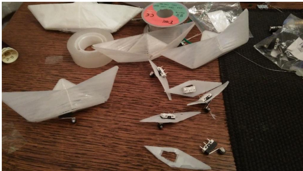
Figure 6-13 The small 3D printed boats with roller switches attached to the bottom
