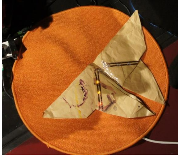
Figure 6-16 Paper butterfly with sticker LEDs and copper tape used inside the dome
