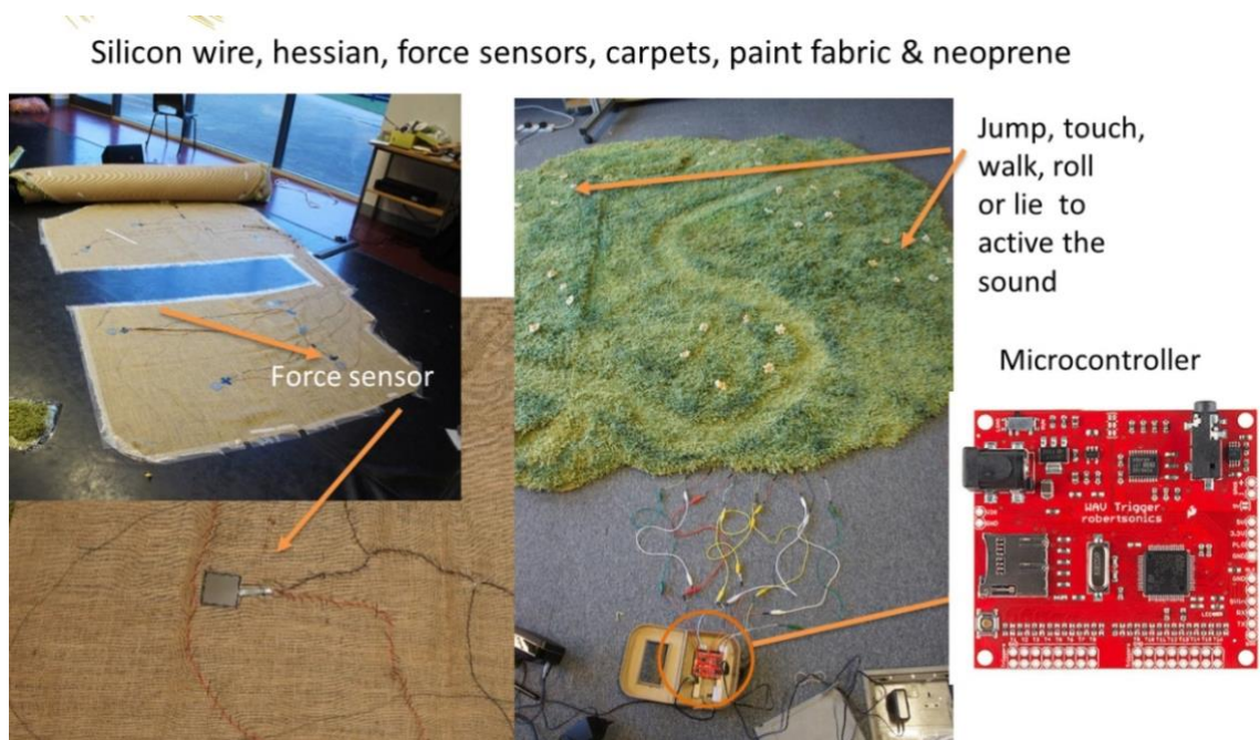
Figure 6-12 The musical meadow force sensors mat and microcontroller Wav Trigger
