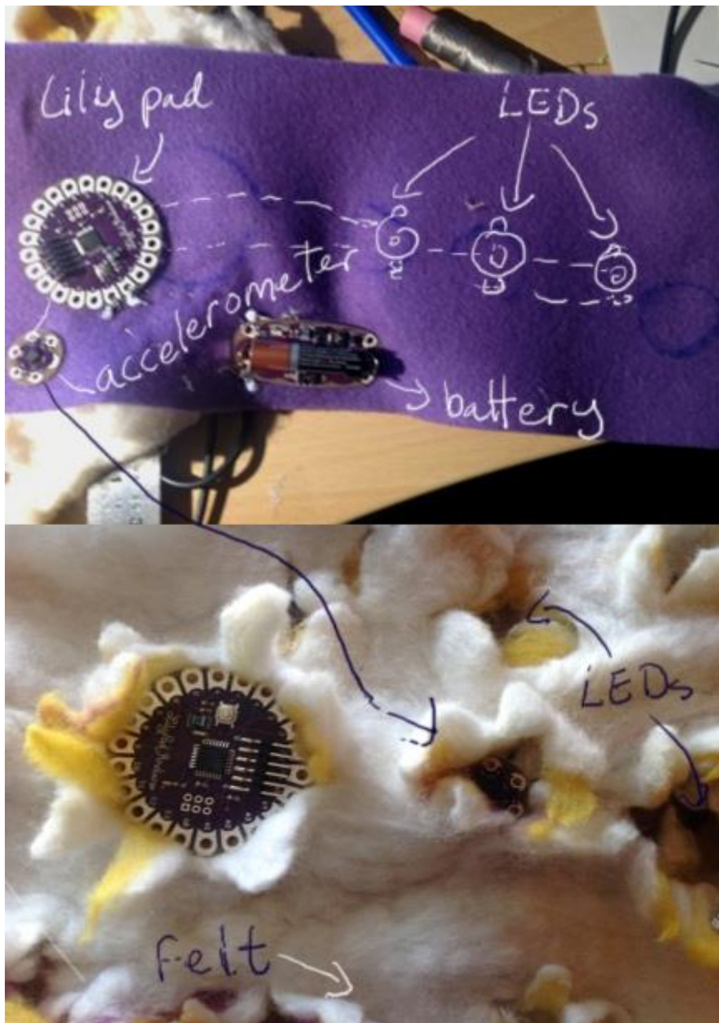
Figure 4-12 Work in progress, the felt caterpillar used wearable technologies – lily pad microcontroller (mini-computer), accelerometer and LEDs.
