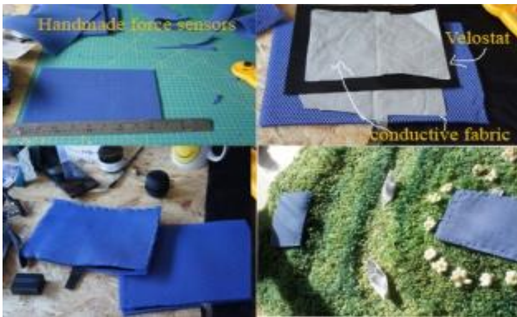
Figure 6-11 Fabric handmade sensors prototype design
