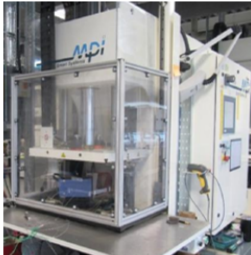
Figure 3.16: Picture of the injection moulding machine used in the conducted experiments.
