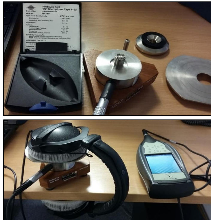
Figure 7: Set up of artificial ear for calibration of sound level of simulations. Top photograph demonstrates the artificial ear and microphone used. Bottom photograph shows the headphones placed over the artificial ear during sound calibration.
