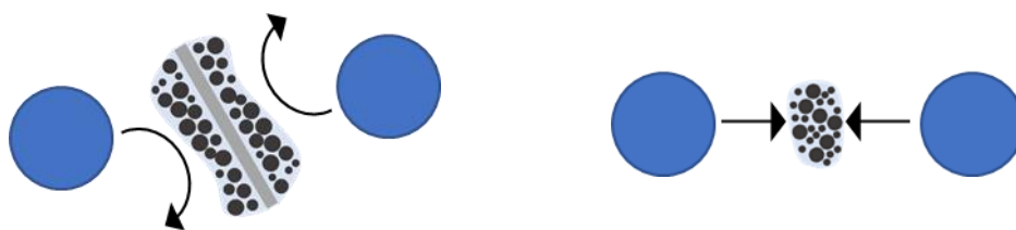
Figure 5-2 The hypothesis of silica sand media on different particle morphology of dry milled LIBs in attrition scrubber; size fraction of > 850 \mu\text{m} (left) and size fraction of < 850 \mu\text{m} (right) with the silica sand media represented by the circles.
