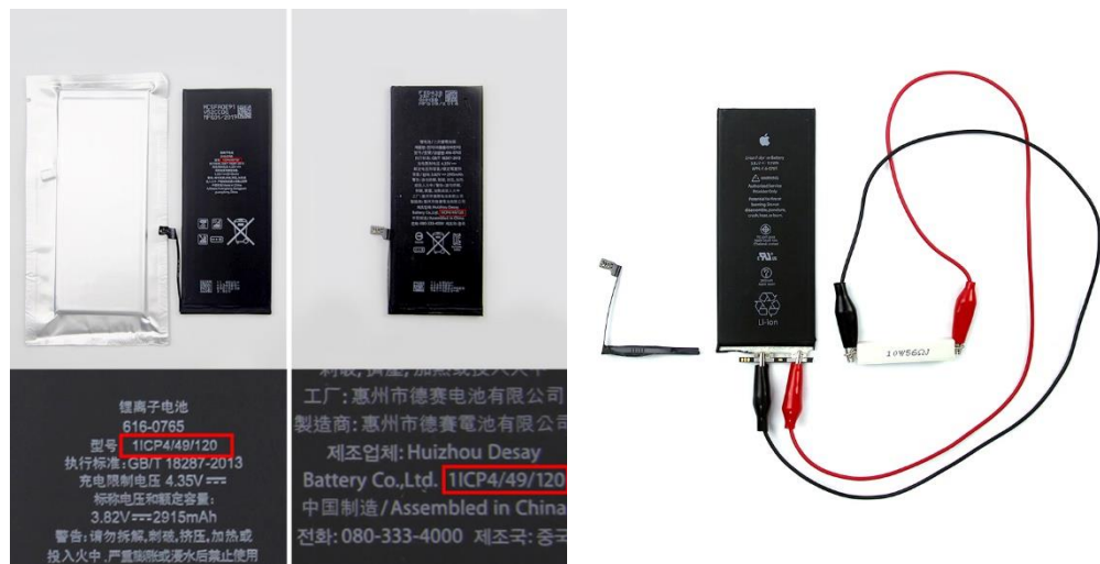
Figure 3-6 Photograph of new ICP-LIBs and spent ICP-LIBs (left); and an example of battery discharging (right).
