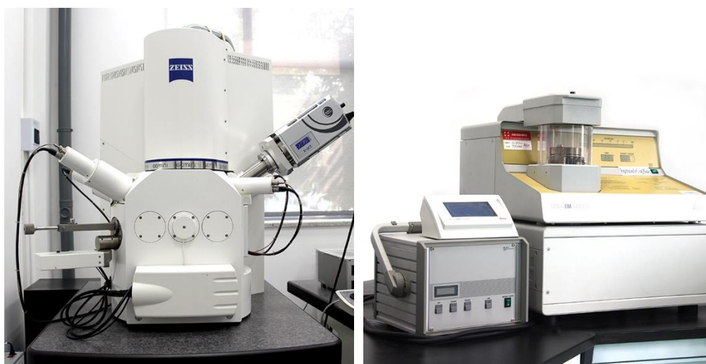
Figure 3-12 Photograph of the Field Emission Scanning Electron Microscopy (FESEM) and equipped with an Energy Dispersive X-Ray (EDX) (left); and the gold sputtering machine (right).
