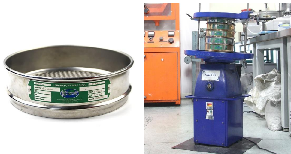
Figure 3-9 Photograph of the certified test sieve (left) and stacked sieves on a sieve shaker (right).
