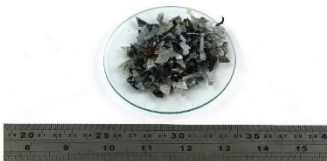
Fig. 3. Classified milled spent LIBs; 3.1) 13200 \mu\text{m} –9500 \mu\text{m} , 3.2) 9500 \mu\text{m} –6700 \mu\text{m} , 3.3) 6700 \mu\text{m} –4750 \mu\text{m} , 3.4) 4750 \mu\text{m} –2360 \mu\text{m} , 3.5) 2360 \mu\text{m} –850 \mu\text{m} , 3.6) 850 \mu\text{m} –212 \mu\text{m} , 3.7) 212 \mu\text{m} –38 \mu\text{m} , 3.8) <38 \mu\text{m} .
