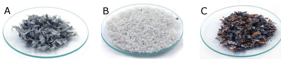
Figure 6-4 Photograph of the electrostatic separation products; A: non-conductor, B: middling, C: conductor.
