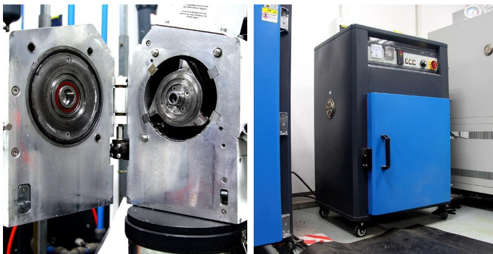
Figure 3-7 – Photograph of cutting mill (left) and the box oven (right).
