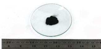
Fig. 3. Classified milled spent LIBs; 3.1) 13200 \mu\text{m} –9500 \mu\text{m} , 3.2) 9500 \mu\text{m} –6700 \mu\text{m} , 3.3) 6700 \mu\text{m} –4750 \mu\text{m} , 3.4) 4750 \mu\text{m} –2360 \mu\text{m} , 3.5) 2360 \mu\text{m} –850 \mu\text{m} , 3.6) 850 \mu\text{m} –212 \mu\text{m} , 3.7) 212 \mu\text{m} –38 \mu\text{m} , 3.8) <38 \mu\text{m} .
