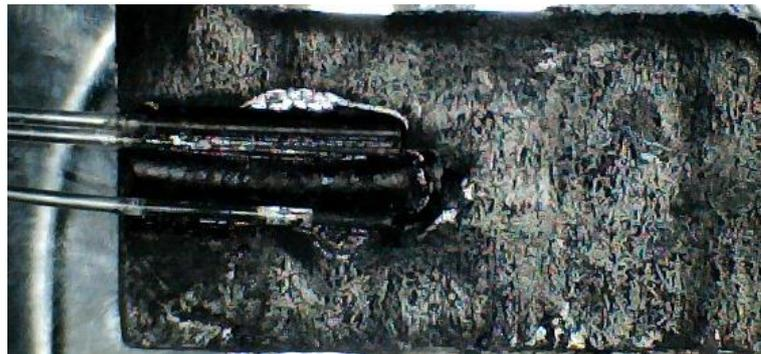
Figure 4.1. (a) The schematic of the POF patch. The patch is a  $20 \times 10 \times 2 \text{ mm}^3$  cube. Three  $45^\circ$  cleaved end POFs are embedded in the slot. The black bar between POFs is used to block light. Red and orange bars present transmit POFs connected to two LEDs (660nm and 850nm). The yellow bar represents the receive POF connected to the photo-diode. (b) The photo of the POF patch.
