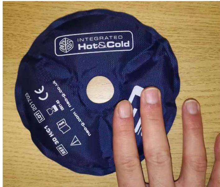
Figure 4.36. Neo G 3D hot&cold therapy disc. The tested finger (index finger) and the reference finger (middle finger) are located on the therapy disc during the cooling process.
