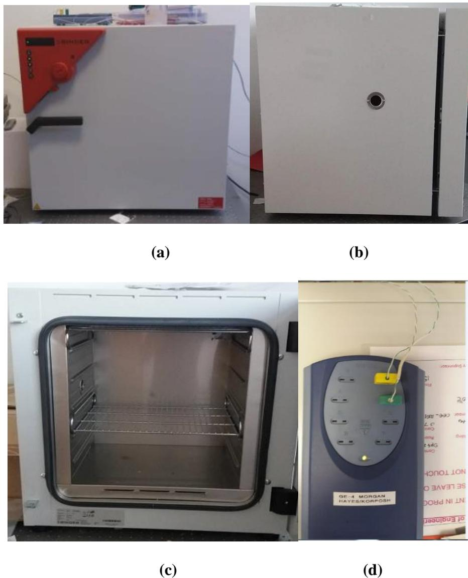
Figure 3.10. Temperature controlling system. (a) Front view of the Binder ED-115 Oven (b) Side view of the oven (c) Inner side of the Binder ED-115 Oven. (d) Pico TC-08 thermocouple logger
