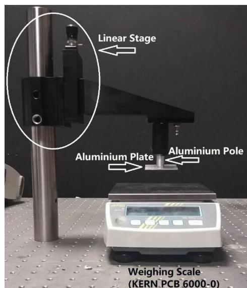
Figure 3.16. Pressure loading system. The manual plate is applied to lift/lower the aluminium pole and plate to load the pressure transversely. The weighing scale beneath records the pressure applied.
