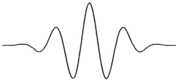
Figure 2.24. The product of a sine wave multiplied by a Gaussian distribution. From DeValois and DeValois (1990).
