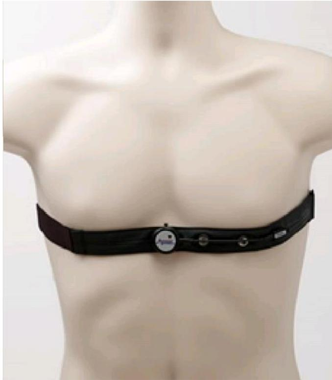
**Figure 2.7.** *An ActiHeart chest belt with an Actiheart monitor attached to measure heart rate and physical activity.*
