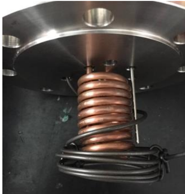
Figure 80 Condenser coil and immersion pre-heater
