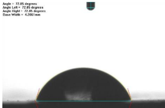
Figure 16 Water static contact angle on uncoated copper surface
