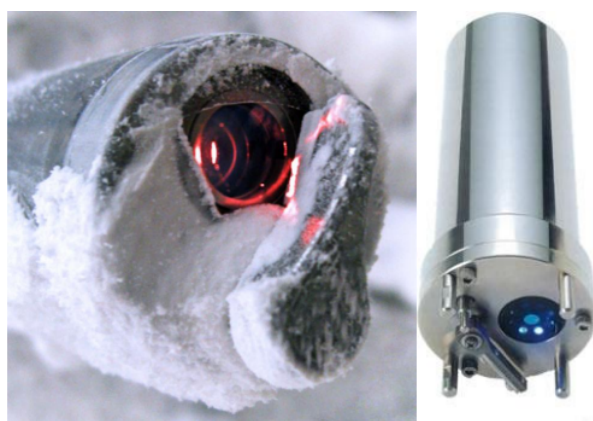
Figure 77: (left) Mechanical scrapper at the tip of a commercial ParticleTrack FBRM C35 probe and an Infinity CLW fluorescence/turbidity/temperature immersion probe [133].
