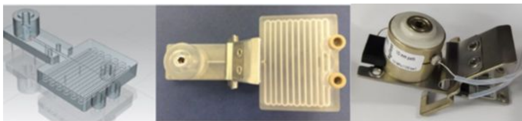
Figure 15: 123x67x47mm CAD model of VP flow reactor (left) Reactor device with sprung clip (centre) commercially available Agilent flow cell (right) [6]
