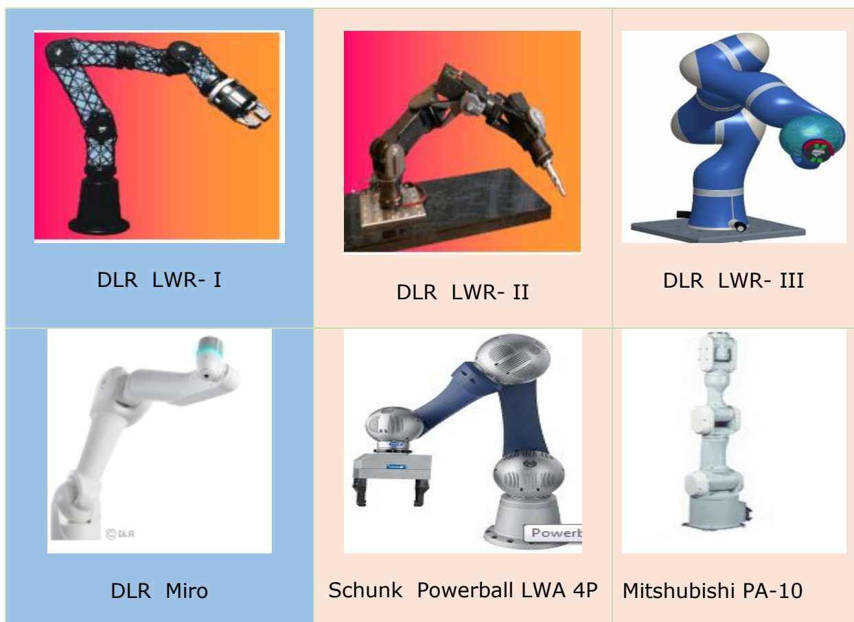
Figure 2.14: Lightweight manipulators designed with modular mechatronic approach.
