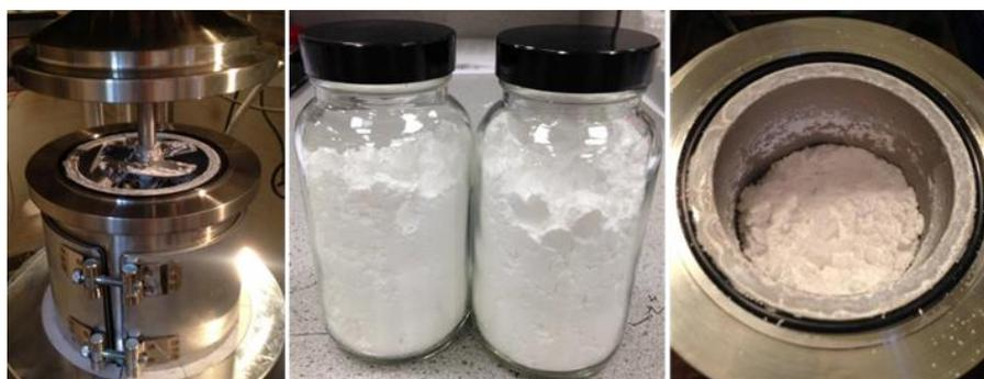
**Figure 4-17: Images showing the product collected from the first MMA polymerisation in the 1 L autoclave. 150 g of free flowing PMMA was produced.**
