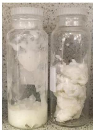
**Figure 3-46: Images of sample produced from synthesising PBzA followed by addition of MMA. The soft nature of PBzA means that the particles are prone to aggregation, preventing formation of stable particles in the first stage of the reaction.**
