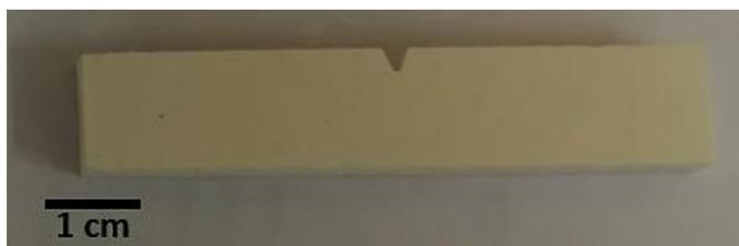
**Figure A-17:** Image showing the single notched test specimens used for the Izod impact testing.
