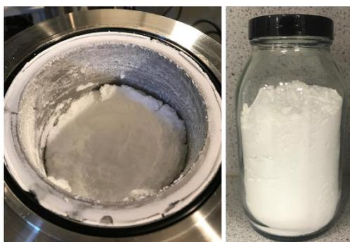
**Figure 4-37: Images showing the free-flowing powder produced in the 1 L autoclave from a reaction where PMMA particles were synthesised before the addition of BA (27 wt%). A yield of 142 g of free flowing white powder was obtained.**
