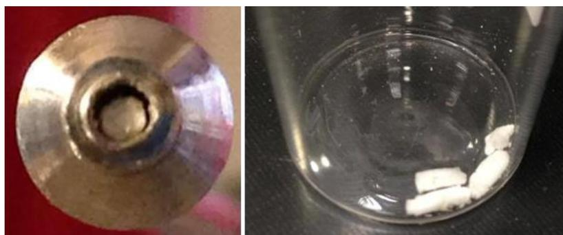
**Figure 4-19: Images of PMMA pellets discovered when cleaning the 1 L autoclave. Left hand image is a face on image of a blocked pipe (CO<sub>2</sub> outlet), right hand image shows PMMA pellets removed from several pipe joints.**
