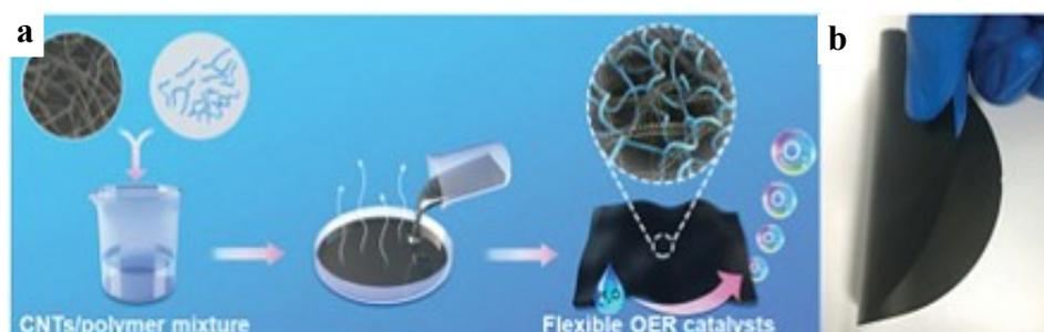
**Fig. 2-8 (a) Schematic illustration of preparation procedure for flexible OER electrocatalyst based on polymer @MWCNTs composite membranes, (b) a photograph of the flexible free-standing PEMAs @MWCNTs 90 membrane. Cited from Ref (Zhang et al. 2017b).**
