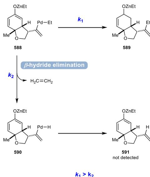
Scheme 84. Reductive elimination is faster than  $\beta$ -hydride elimination on this process.
