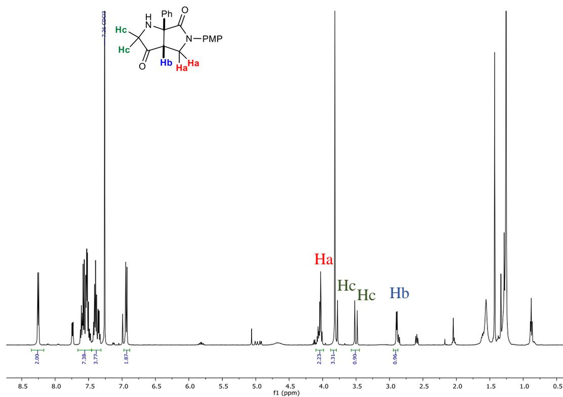
Chemical shifts of the distinctive protons are consistent with the structure. Both diastereotopic protons **Ha** next to an electronegative amidic nitrogen (around 4 ppm); **Hc** next to an electronegative nitrogen and a carbonyl (around 3.5 ppm) and **Hb** next to a carbonyl (between 2 and 3 ppm).
