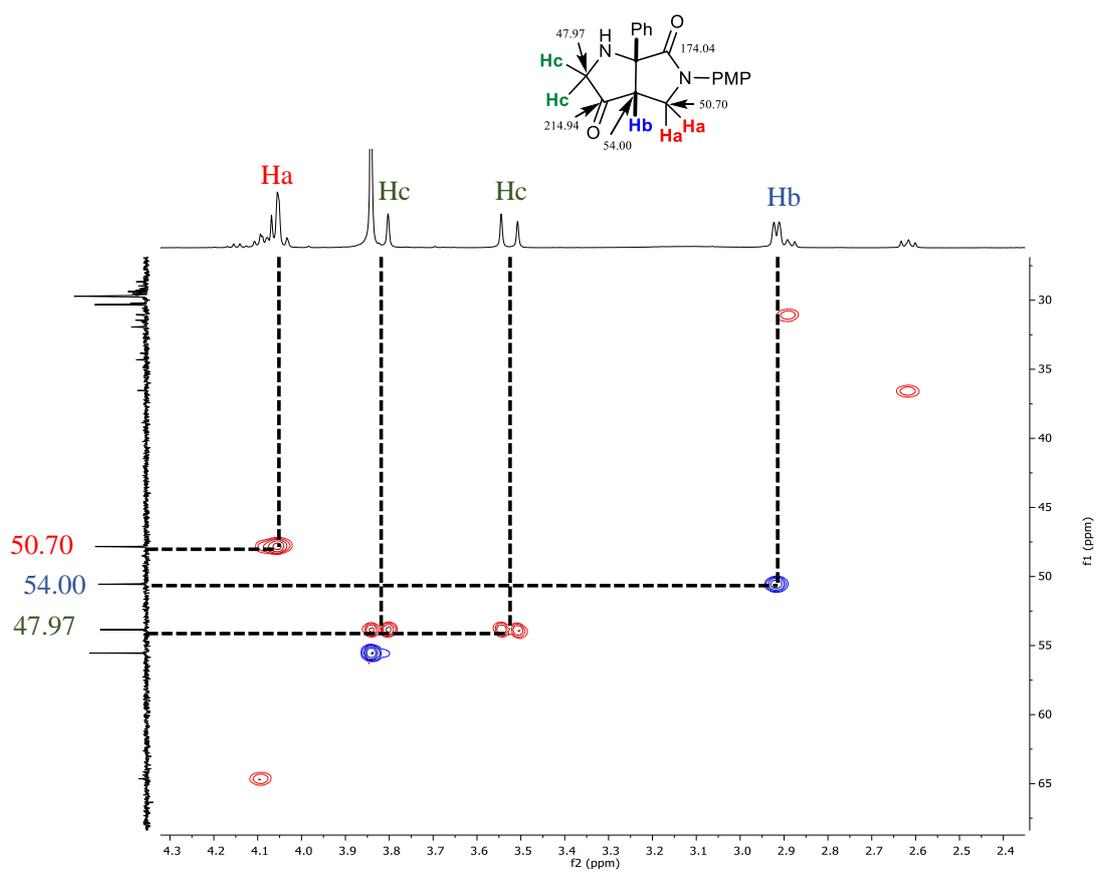
With the HSQC spectrum it is possible to assign the signals of the carbons bearing the distinctive protons.
