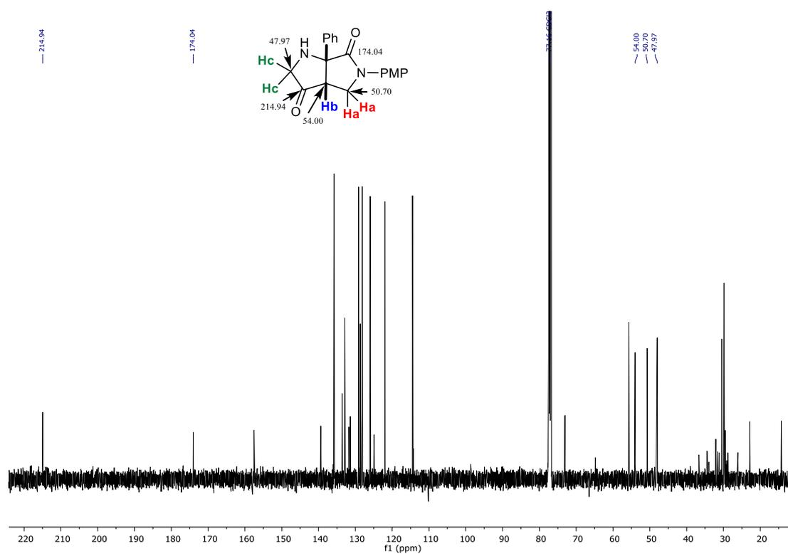
Highlighted are the distinctive peaks of the structure: 214.9 (C=O in a five-membered ring); 174.0 (C=O of a  $\gamma$ -lactam); Ha, Hb and Hc between 40 and 60 ppm, consistent with the shifts of aliphatic  $^{13}\text{C}$  next to electronegative functional groups. Analysis of HSQC spectrum helped in assign the peaks.
