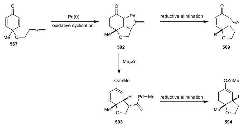
Scheme 85. Possible mechanism with Pd(0).
