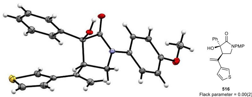
Figure 2 compound **516** X-ray crystallography reveals absolute and relative stereochemistry of this compound.
