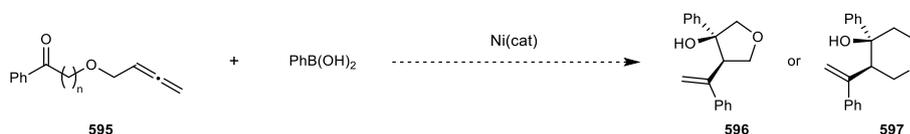
Scheme 86. Future work ongoing with regard to the expansion of the substrate scope.
