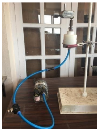
Figure 2.9 Cyclone and filter holder assembly for the collection of PM 2.5 from the combustion of biomass fuel.
