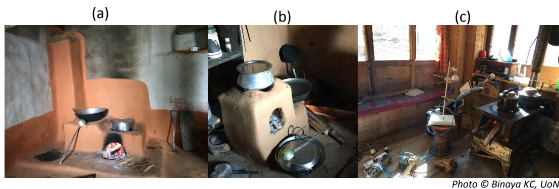
Figure 1.16 Improved cook stove (ICS), commonly used in various regions of Nepal. (a) two pot mud ICS, (b) single pot mud ICS and (c) two pot metallic ICS.
