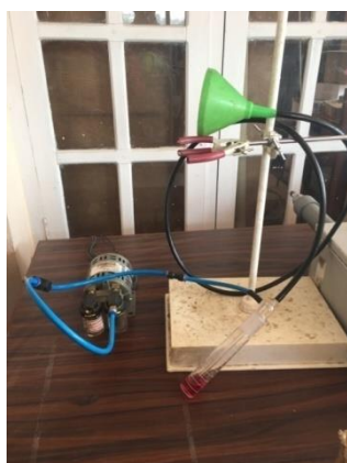
Figure 2.10. Media based smoke sample collection unit.
