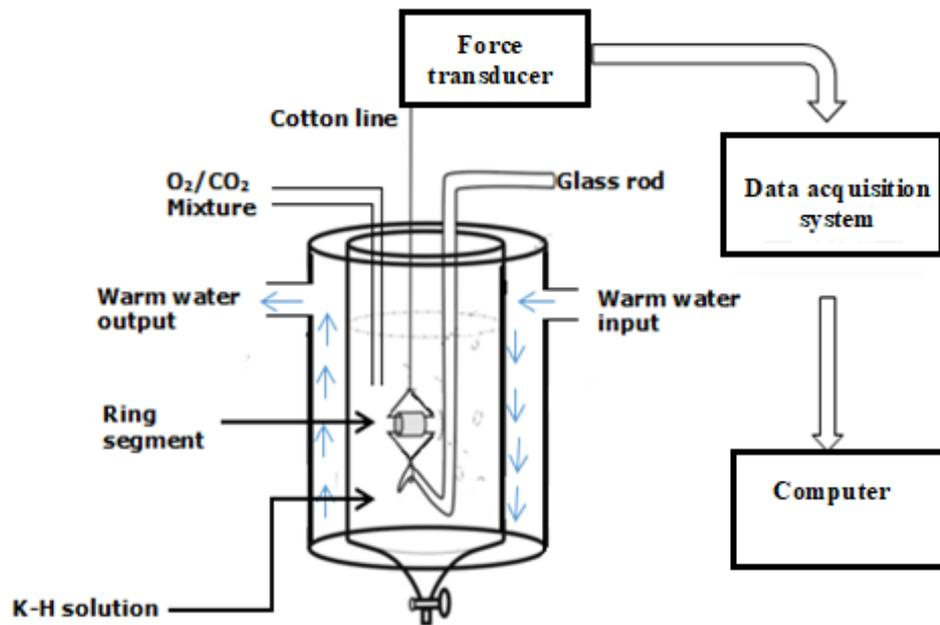
**Figure 2.3 Schematic diagram of the organ bath set-up for porcine blood vessels contractility studies.** Investigated drugs were added into a 20ml organ bath containing warmed (37°C) Krebs-Henseleit buffer solution.
