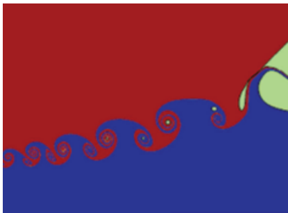
Figure 2.31: Von Karman Vorticity predicted computationally at the droplet-film interface by Thoraval et al. [27]
