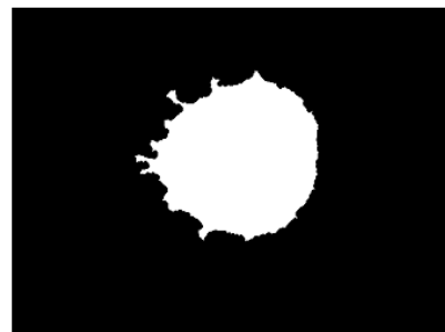
(b) Thresholded to detect droplet material, secondary droplets removed using bwareaopen
