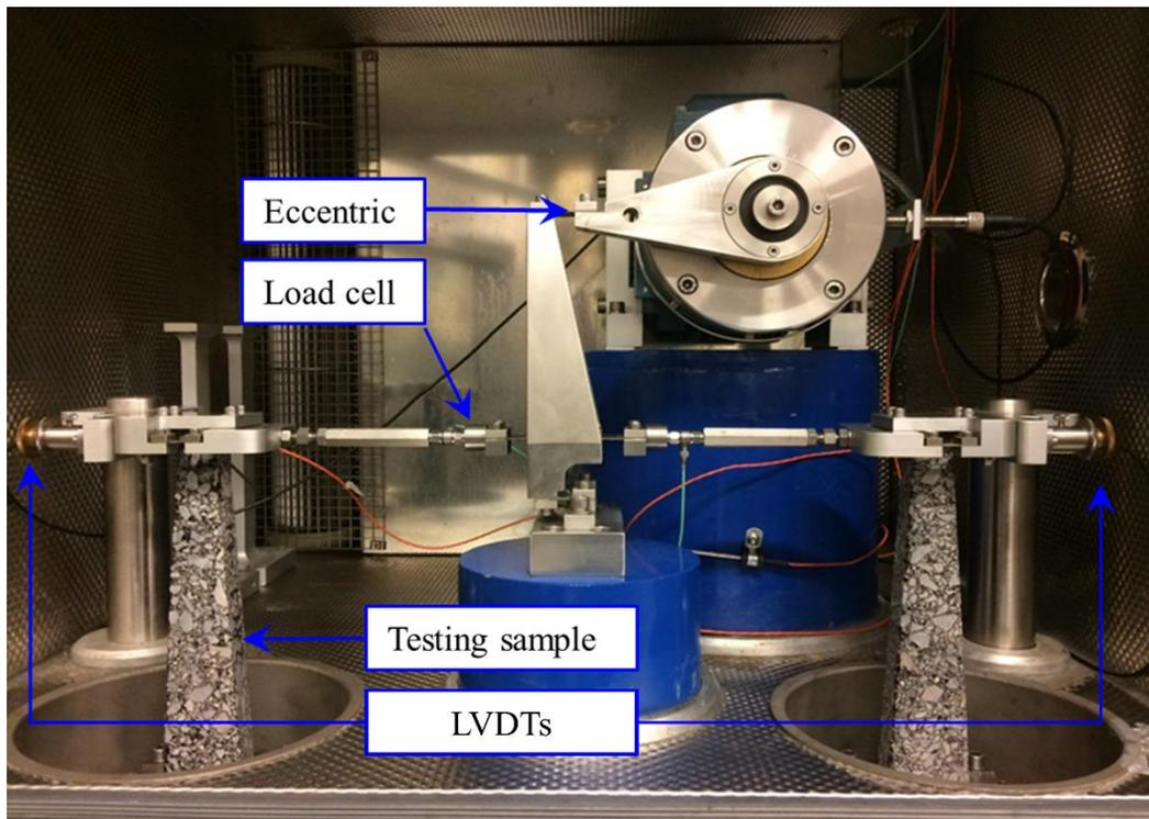
Figure 6-2. Two-point bending machine
