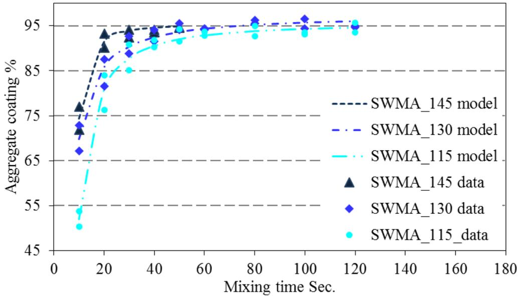
Figure 4-7. Aggregate coating results of SWMA
