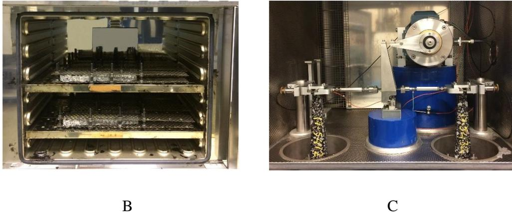
Figure 6-36. LTOA setup for trapezoidal and cylindrical specimens; A, a trap sample sandwiched between two holed plates, B, ageing of trap samples in an oven, and C, testing of trap samples after LTOA process in the two-point bending
