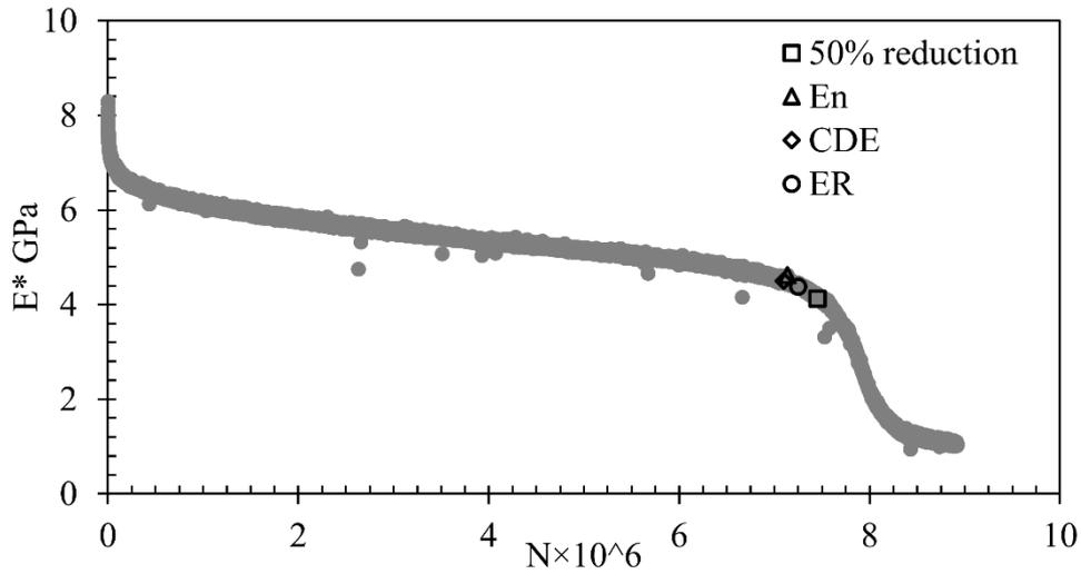
Figure 6-28. WMRA fatigue life determination, at 20°C and 100 με
