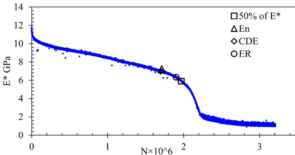
Figure 6-26. SWMA fatigue life determination, at 20°C and 100  $\mu\epsilon$
