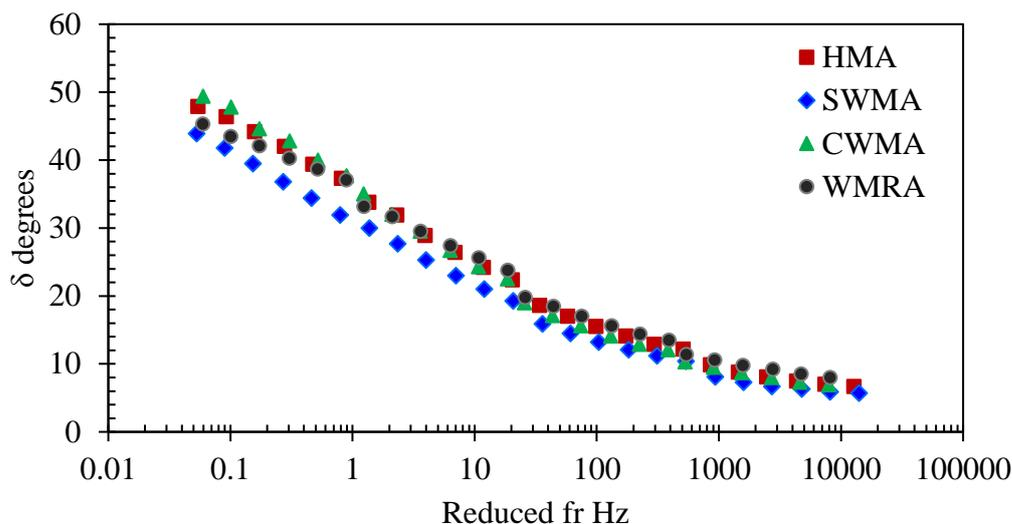
Figure 6-8. Phase angle master curves of the studied mixes
