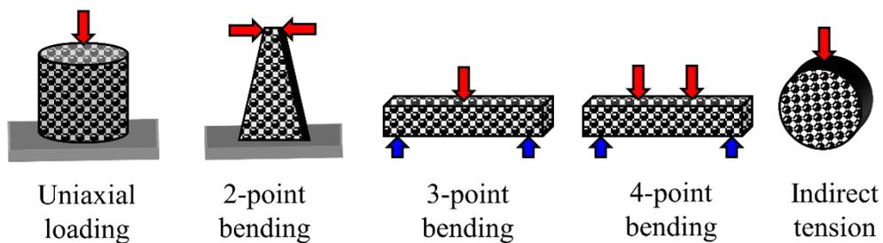
Figure 6-19. Asphalt fatigue cracking testing configurations
