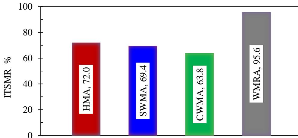
Figure 6-46. ITSMR results after moisture conditioning
