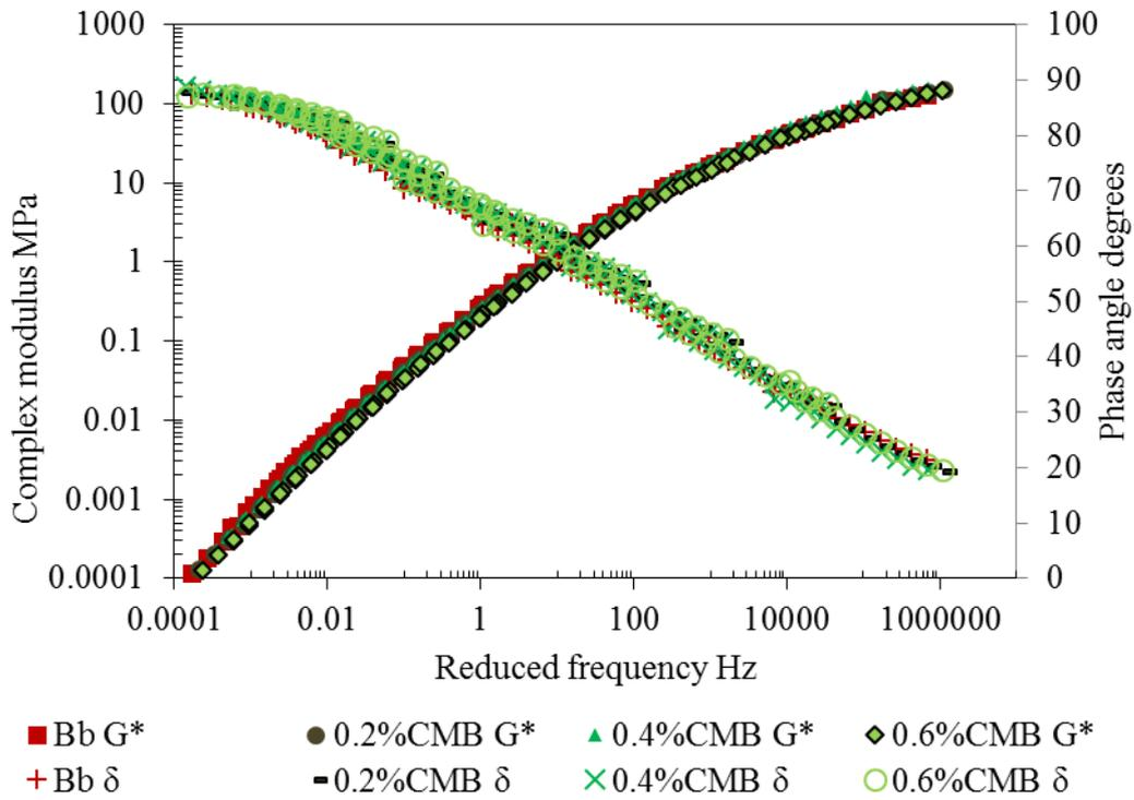
Figure 3-22. G\* and  $\delta$  results of CMBs after RTFOT+PAV ageing
