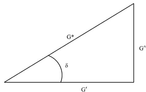
Figure 3-9. Phase angle, storage modulus, loss modulus, and shear modulus relationship
