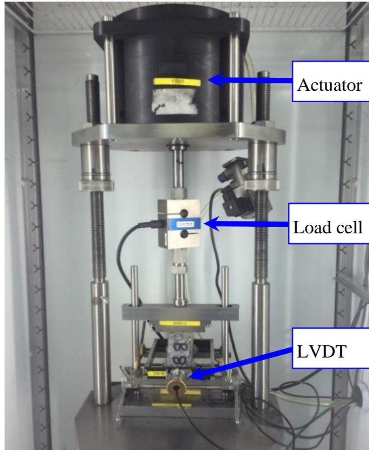
Figure 4-12. Nottingham Asphalt Tester
