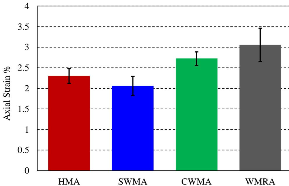
Figure 6-13. RLAT results at 50°C and 3600 load application
