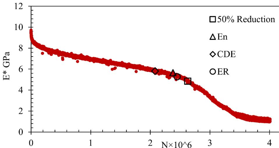
Figure 6-25. HMA fatigue life determination, at 20°C and 100  $\mu\epsilon$
