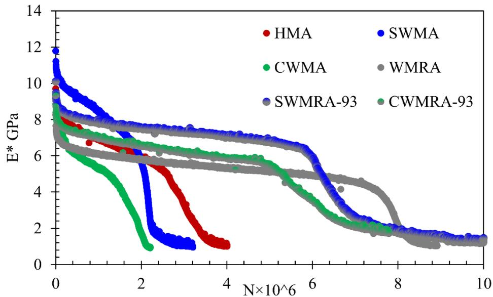
Figure 6-31. Fatigue curves of all mixtures at 20°C and 100  $\mu\epsilon$
