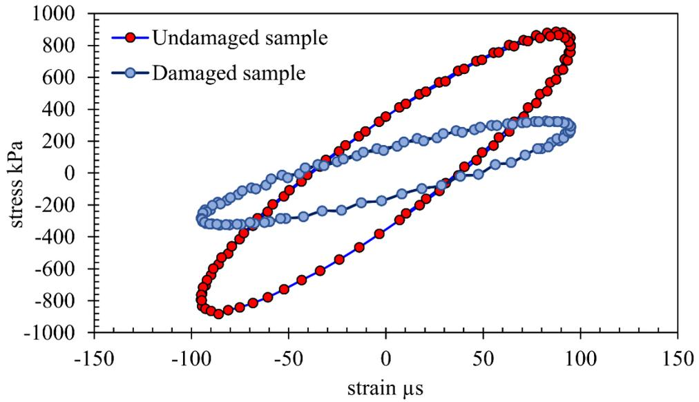
Figure 6-22. Hysteresis loops of an asphalt sample before and after fatigue damage
