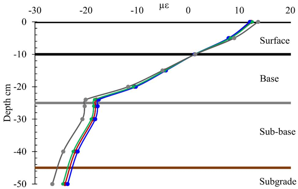
Figure 7-13. Horizontal tensile strain levels in the cold weather
