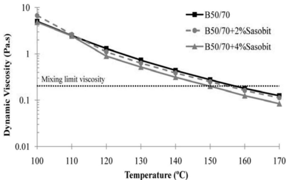
Figure 2-5. Mixing temperature reduction based on the equi-viscous method
