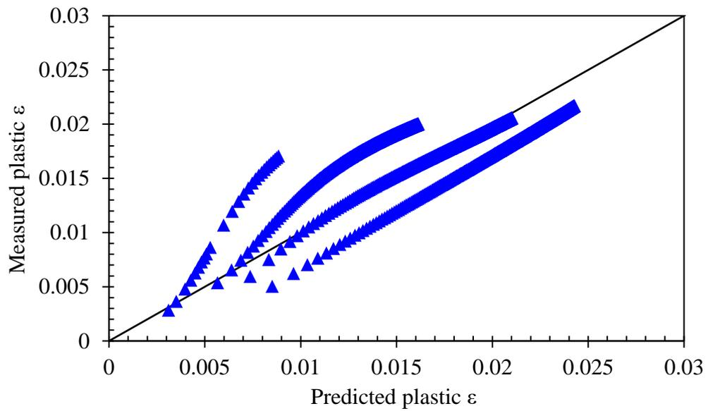
Figure 7-2. Measured and predicted RLAT results of SWMA mix
