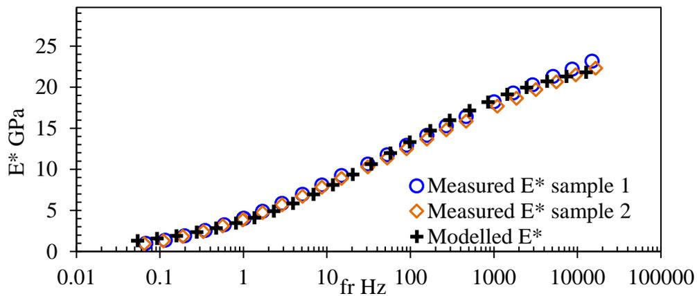
Figure 6-3. E\* master curve of HMA
