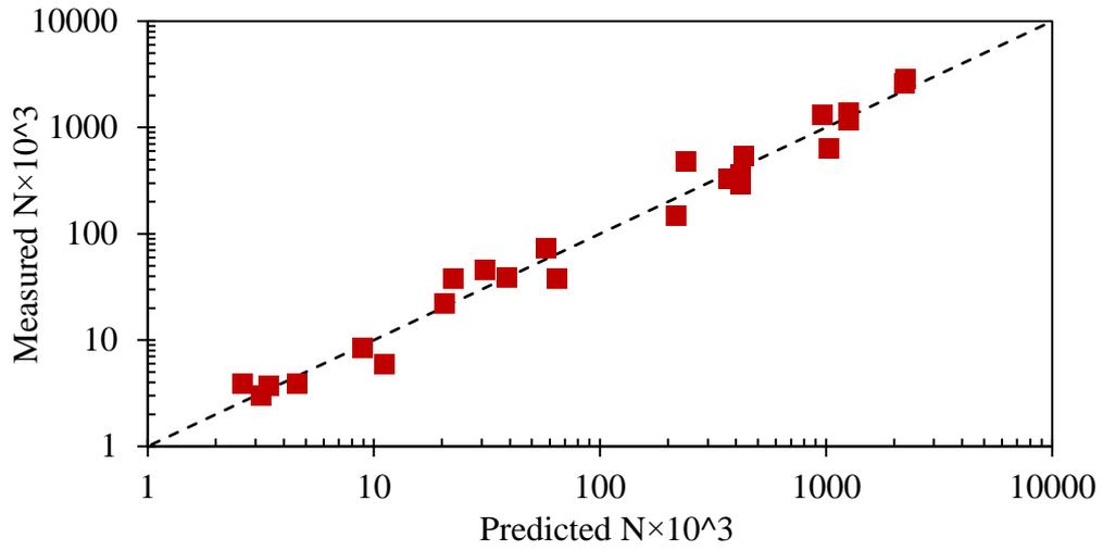
Figure 7-5. Measured versus predicted fatigue life of HMA
