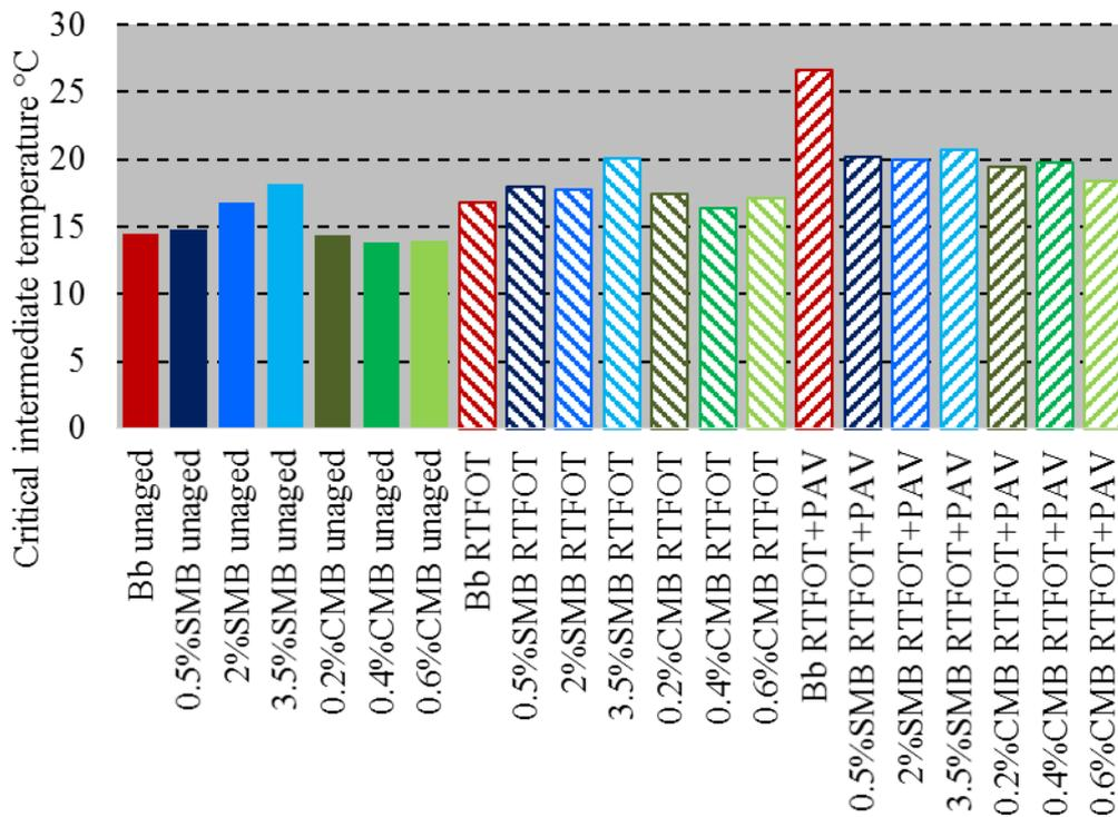
Figure 3-23. Critical intermediate temperatures of the analysed binders
