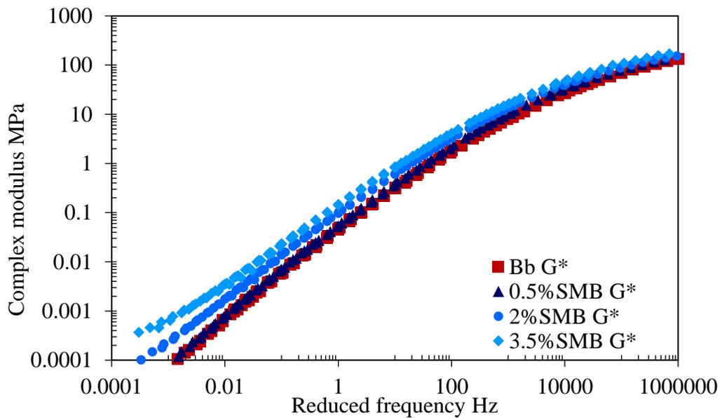
Figure 3-12. Complex modulus master curve for Bb and SMBs
