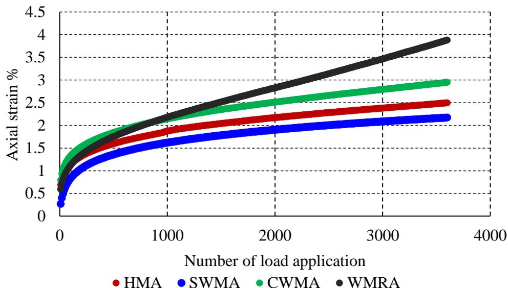
Figure 6-11. Typical RLAT results (at 60°C)
