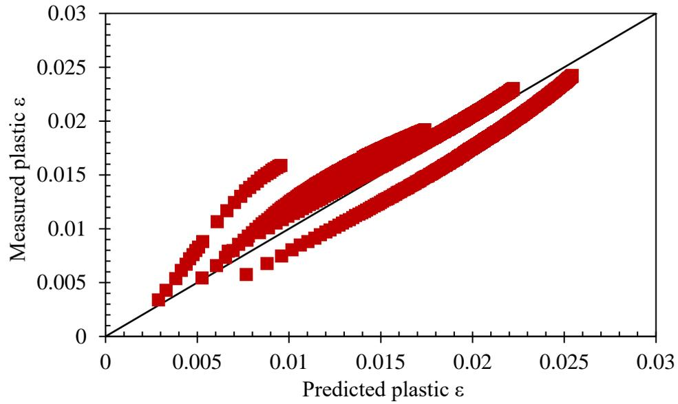
Figure 7-1. Measured and predicted RLAT results of HMA mix
