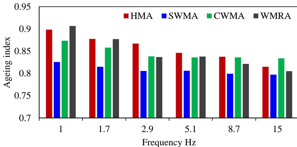
Figure 6-39 Ageing index by  $\delta$  at 30°C
