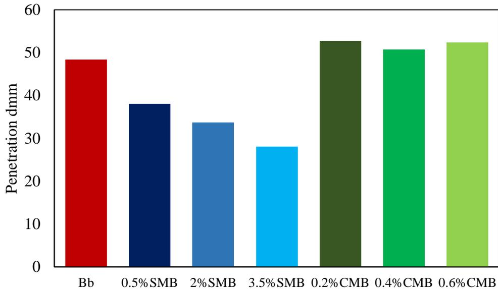
Figure 3-4. Penetration test results
