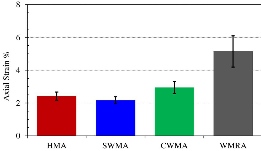
Figure 6-14. RLAT results at 60°C and 3600 load application
