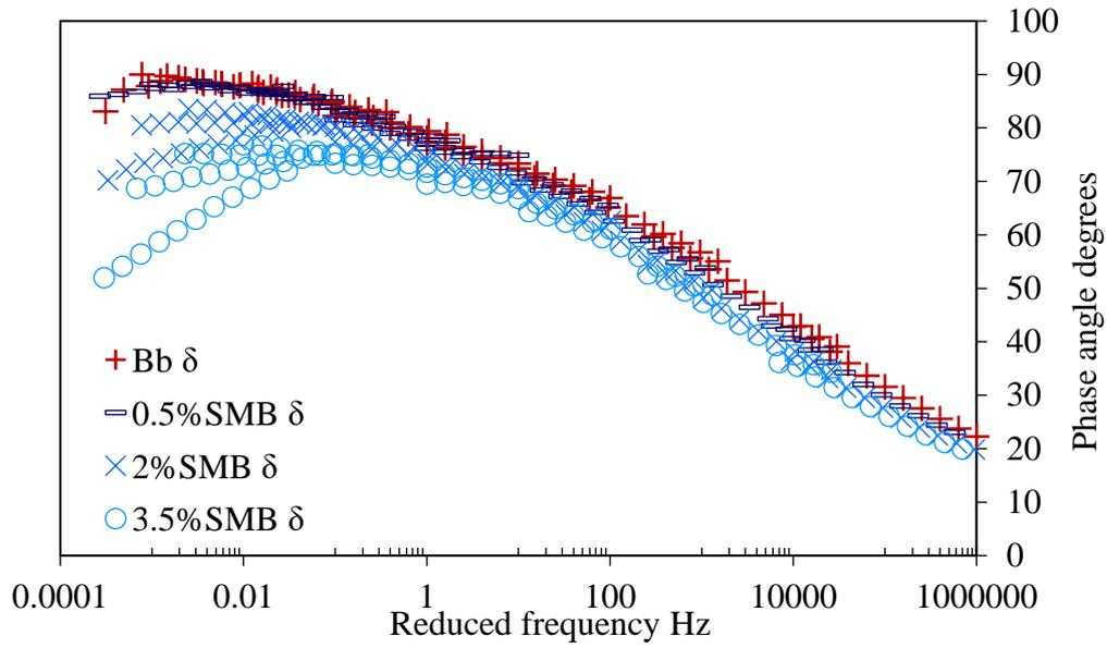
Figure 3-13. Phase angle master curve for Bb and SMBs
