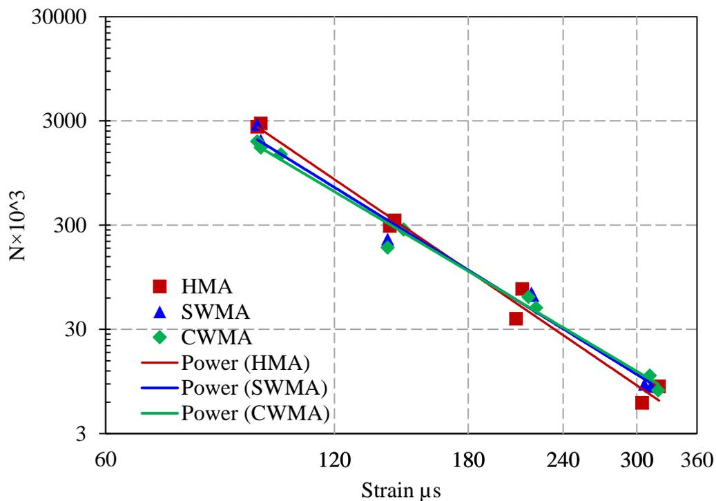
Figure 6-32. Fatigue lines of HMA, SWMA, and CWMA at 20°C
