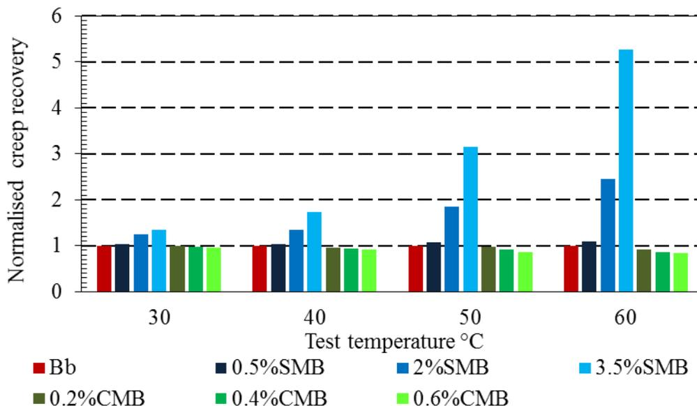
Figure 3-26. Normalised creep recovery results
