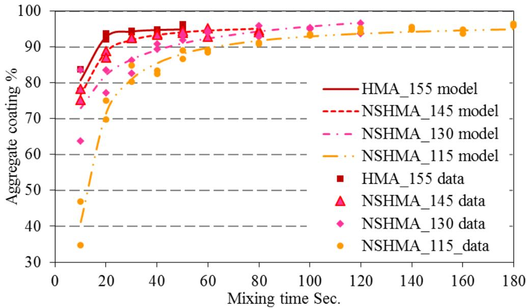
Figure 4-6. Aggregate coating results of HMA and NSHMA
