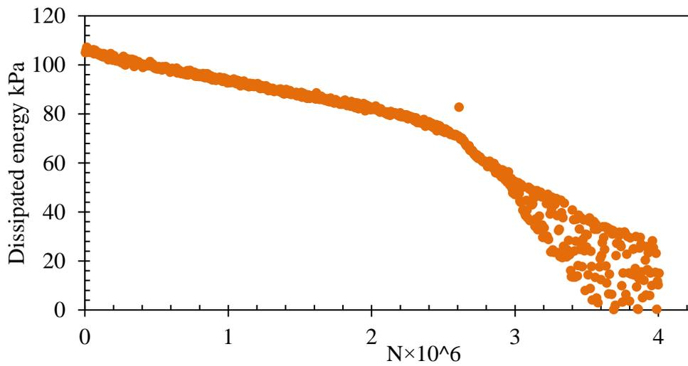
Figure 6-23. Dissipated energy reduction due to fatigue damage
