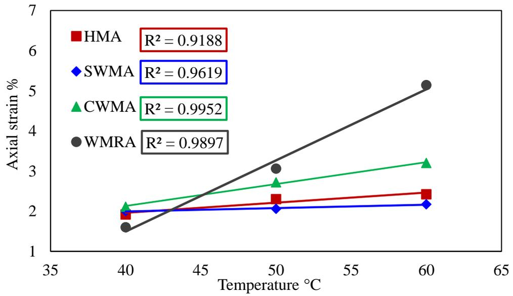
Figure 6-15. RLAT results of all mixtures at 40, 50, and 60°C
