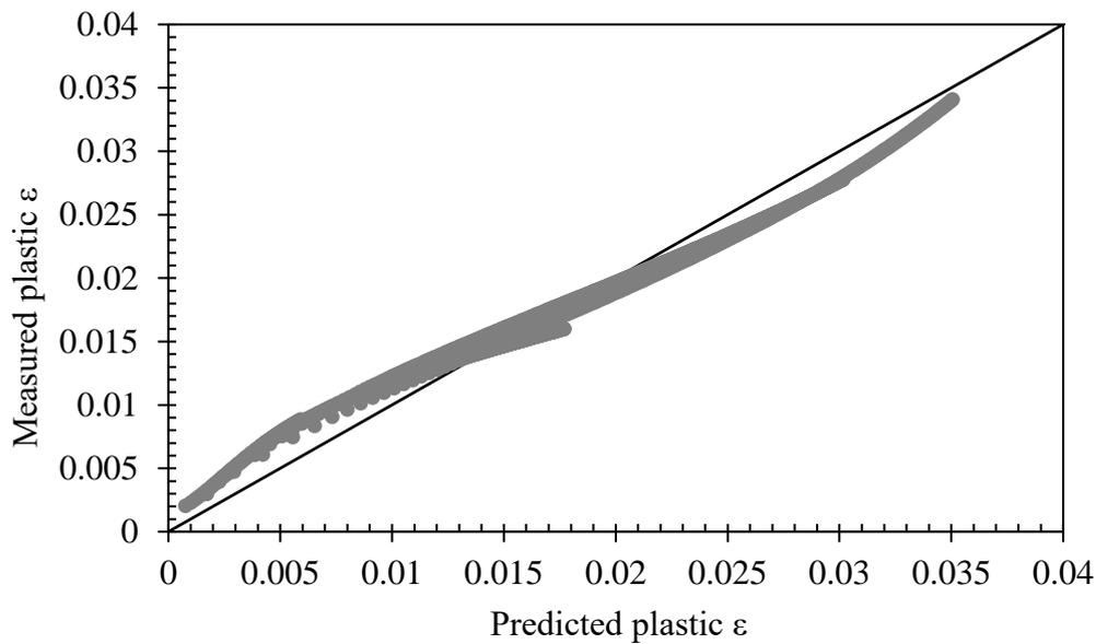
Figure 7-4. Measured and predicted RLAT results of WMRA mix
