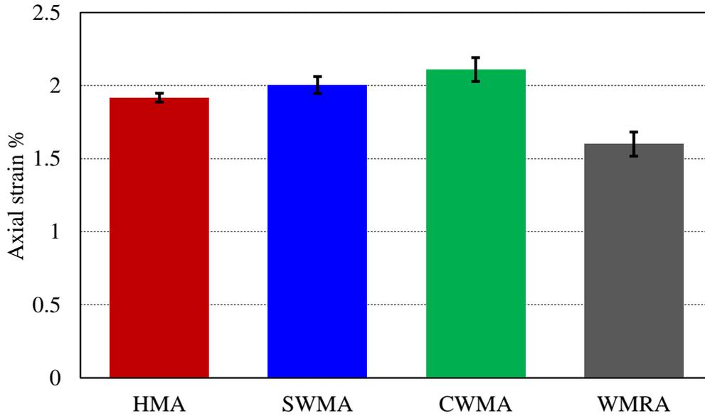
Figure 6-12. RLAT results at 40°C and 3600 load application (error bars represent the minimum and maximum values)
