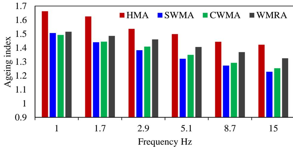
Figure 6-38. Ageing index by  $E^*$  at 30°C
