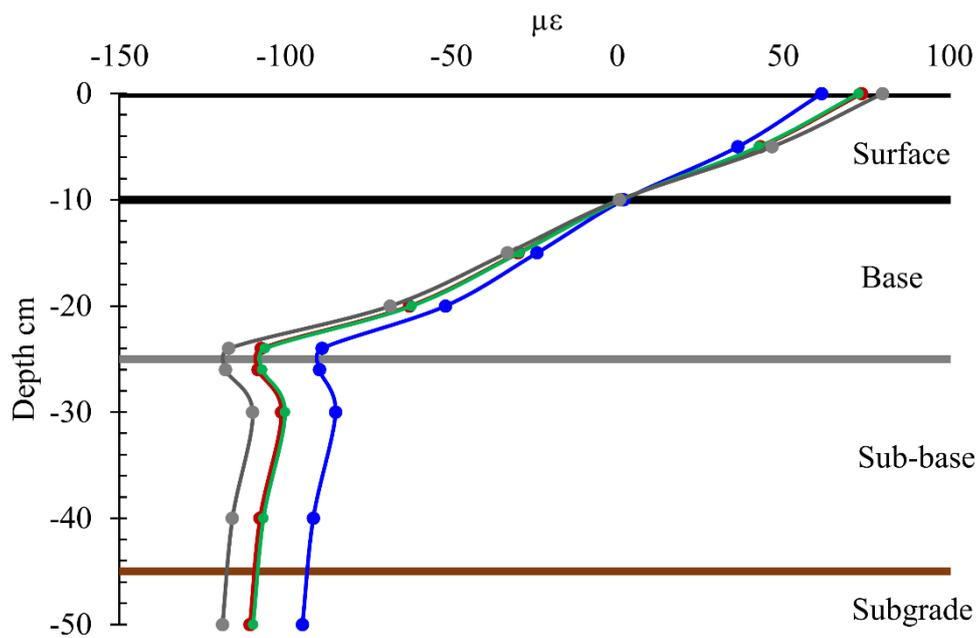
Figure 7-14. Horizontal tensile strain levels in the hot weather
