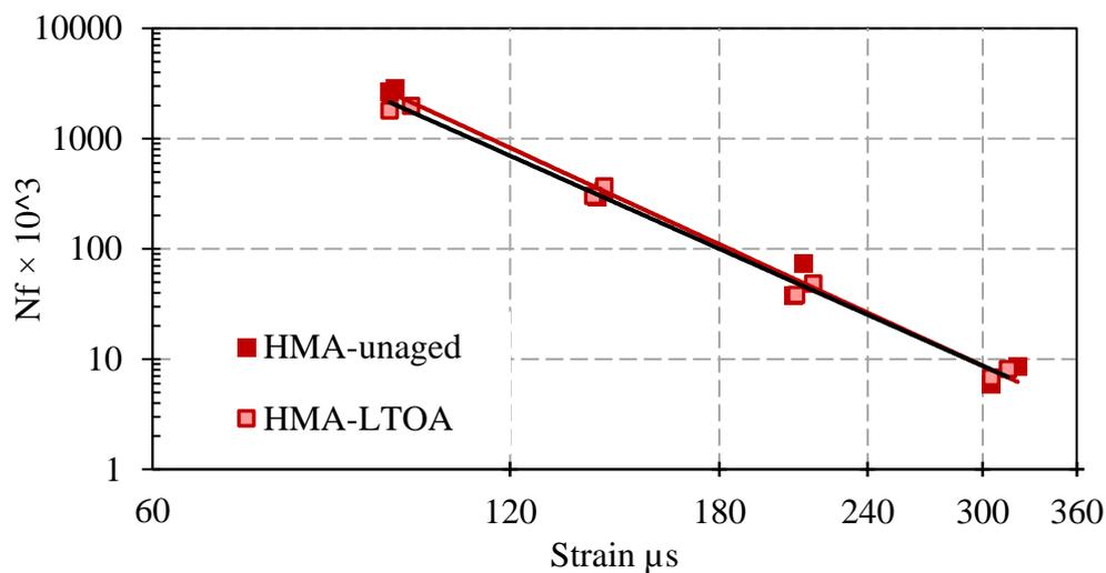
Figure 6-40. Fatigue lines of HMA before and after ageing
