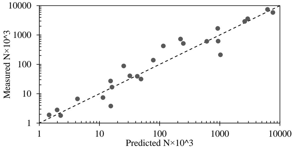
Figure 7-8. Measured versus predicted fatigue life of WMRA
