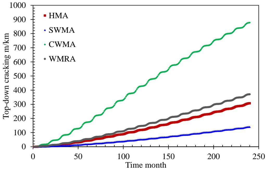
Figure 7-20. Predicted top-down fatigue cracking
