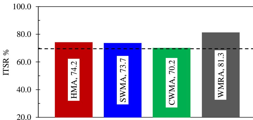
Figure 6-48. ITSR results after moisture conditioning
