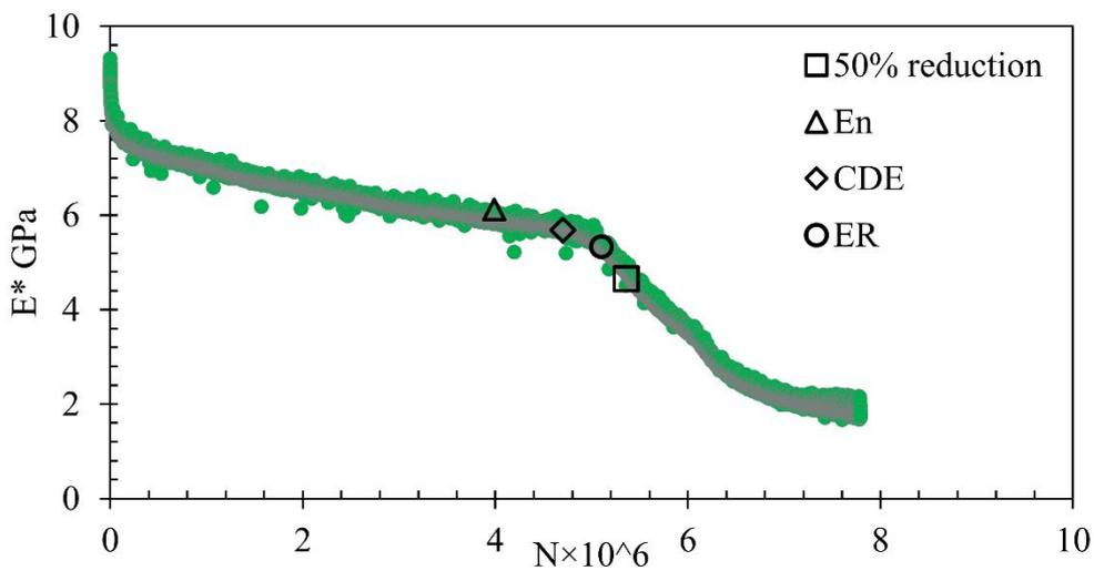
Figure 6-30. CWMRA fatigue life determination, at 20°C and ~100 με
