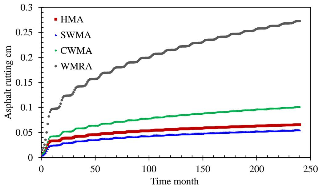
Figure 7-21. Predicted rutting in asphaltic layers
