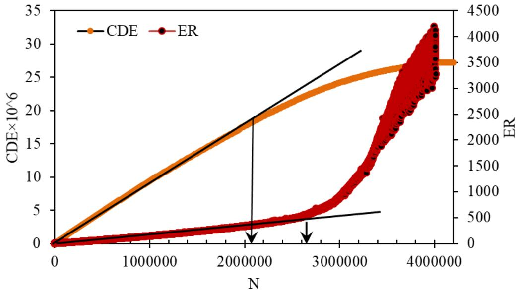
Figure 6-24. Failure definition of CDE and ER methods
