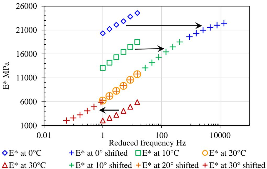
Figure 6-1. Construction of  $E^*$  master curve; reference temperature is 20°C
