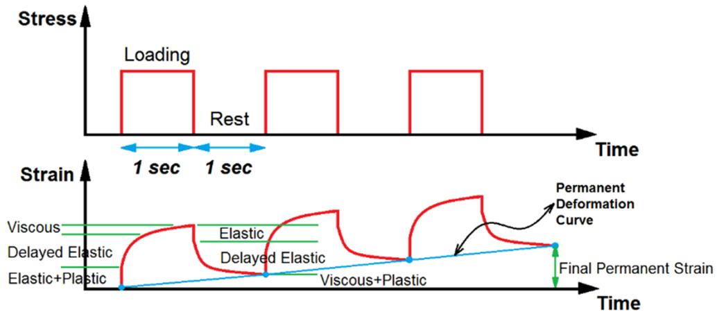
Figure 6-10. Load form and strain accumulation during RLAT (Jalali, 2016)
