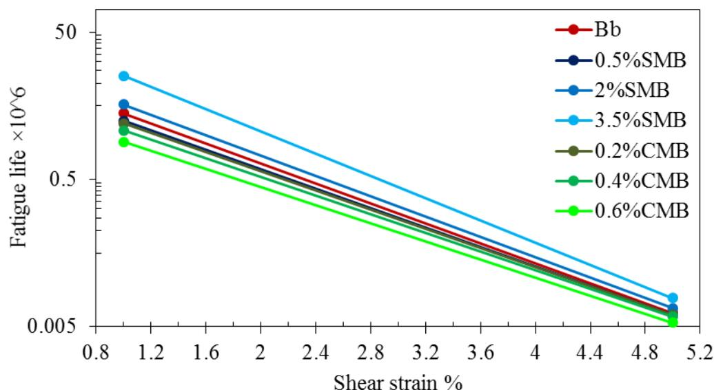
Figure 3-30. Fatigue lines of the studied binders
