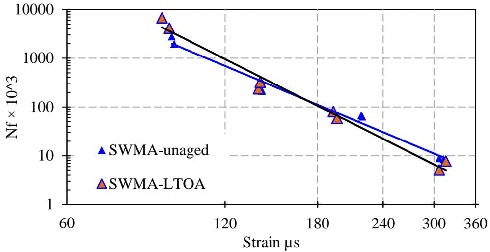
Figure 6-41. Fatigue lines of SWMA before and after ageing
