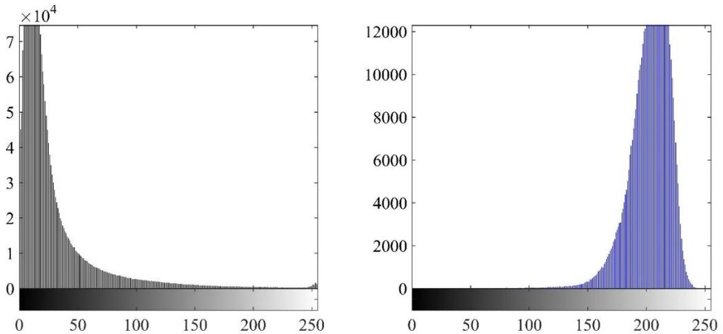
Figure 4-4. Histograms of two images: entirely coated asphalt (left), aggregate only (right)
