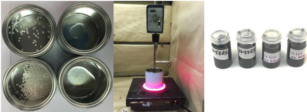
Figure 3-2. Binder modification process
