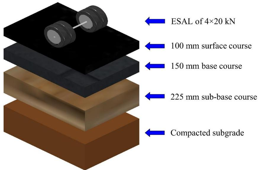
Figure 7-11. Pavement structure considered in the modelling process
