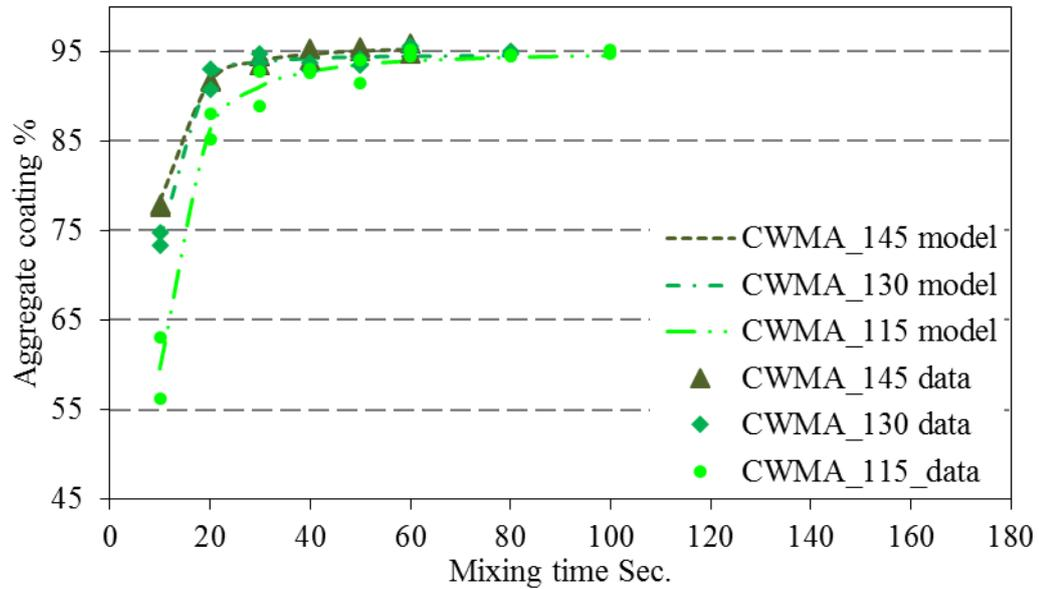
Figure 4-8. Aggregate coating results of CWMA
