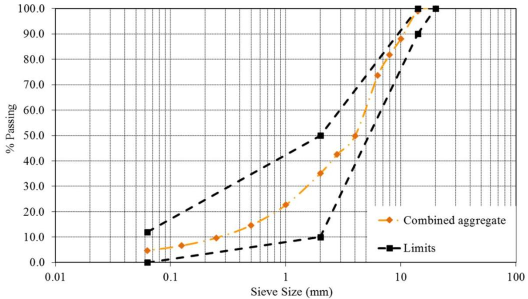
Figure 4-1. AC 0/14mm aggregate gradation
