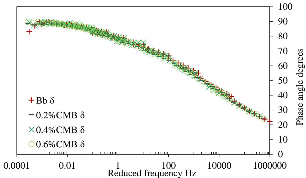
Figure 3-15. Phase angle master curve for Bb and CMBs
