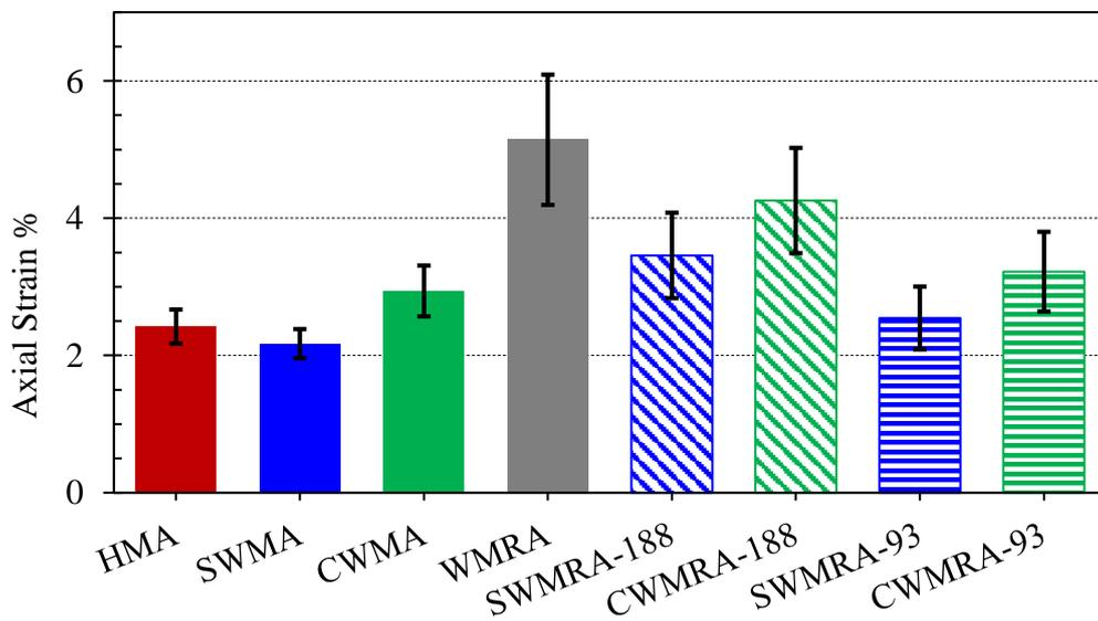
Figure 6-18. RLAT results at 60°C
