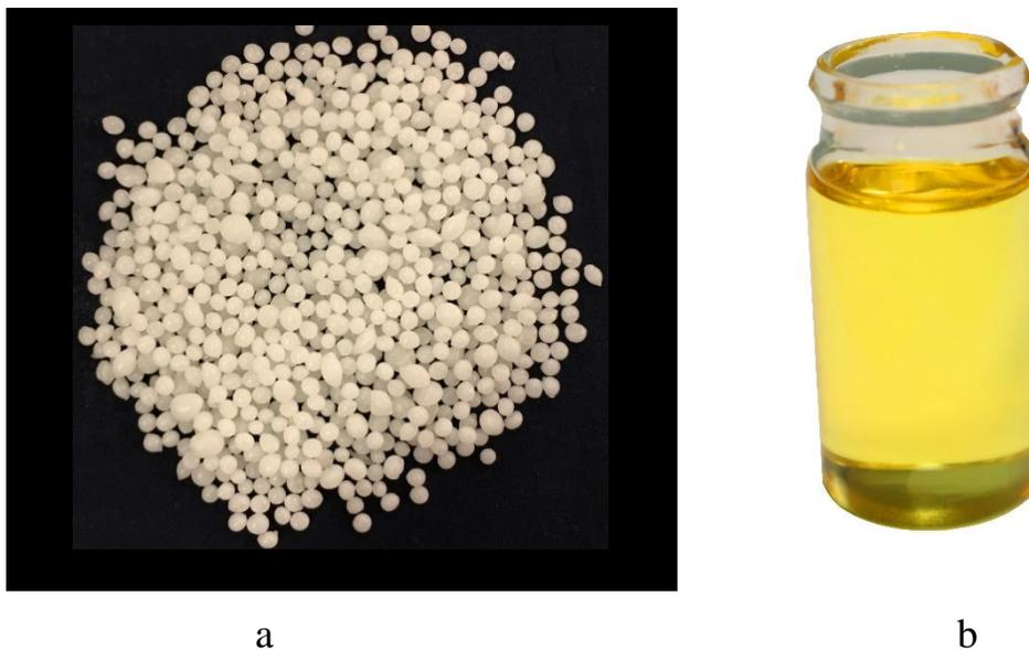
Figure 3-1. WMA additives, (a) Sasobit and (b) Cecabase
