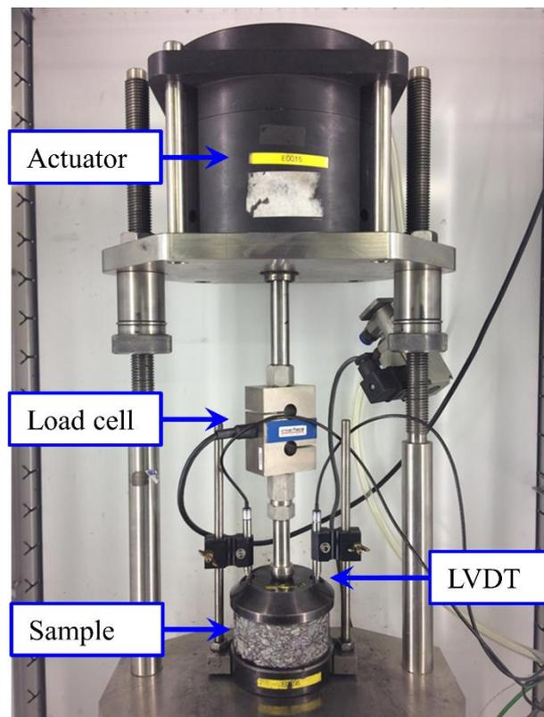
Figure 6-9. RLAT setup using NAT machine
