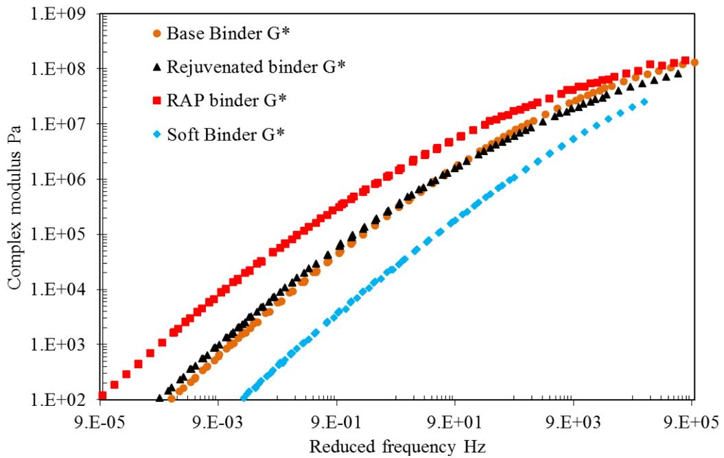
Figure 5-4. Complex modulus master curves
