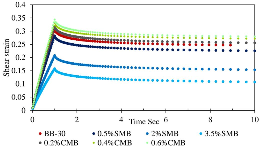
Figure 3-24. Creep and recovery of the studied binders at 60°C and 3.2 kPa loading stress
