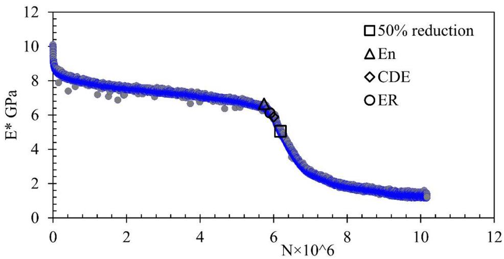
Figure 6-29. SWMRA fatigue life determination, at 20°C and 100 με
