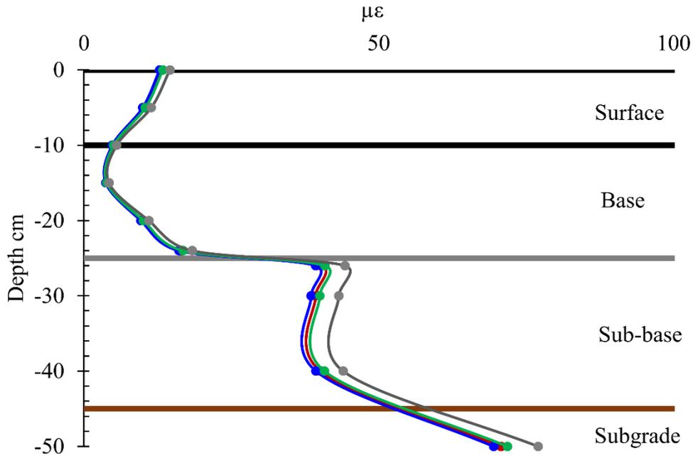
Figure 7-15. Compressive strain levels in the cold weather
