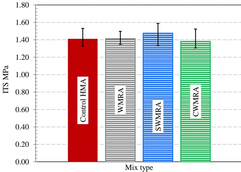
Figure 5-14. ITS results of 50% RAP mixes produced using WMA additives
