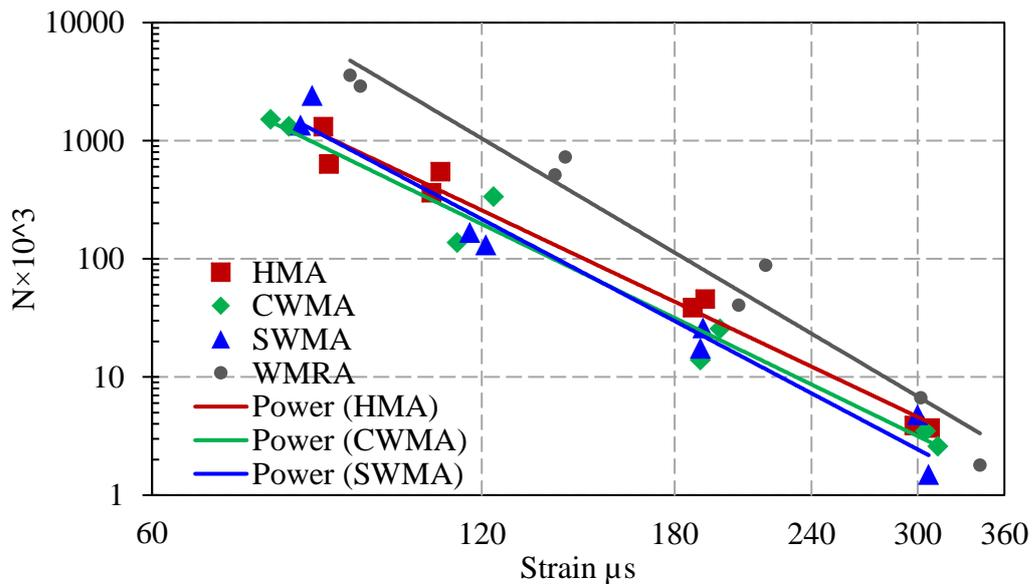
Figure 6-34. Fatigue cracking results at 10°C
