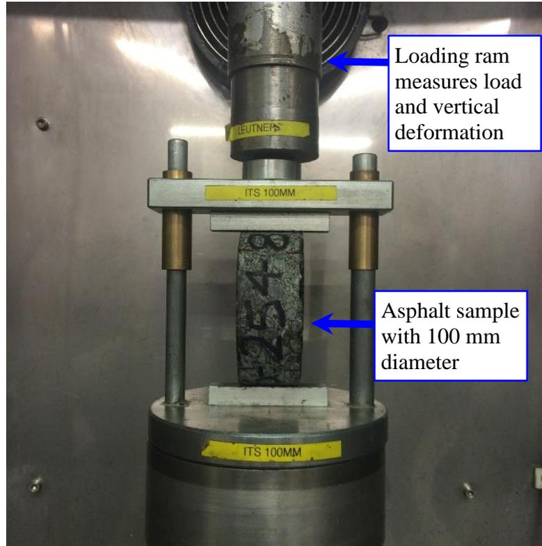
Figure 4-14. ITS test setup
