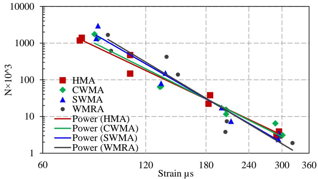
Figure 6-35. Fatigue cracking results at 0°C
