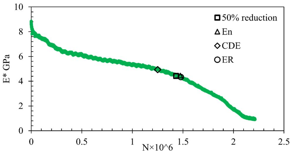
Figure 6-27. CWMA fatigue life determination, at 20°C and 100  $\mu\epsilon$
