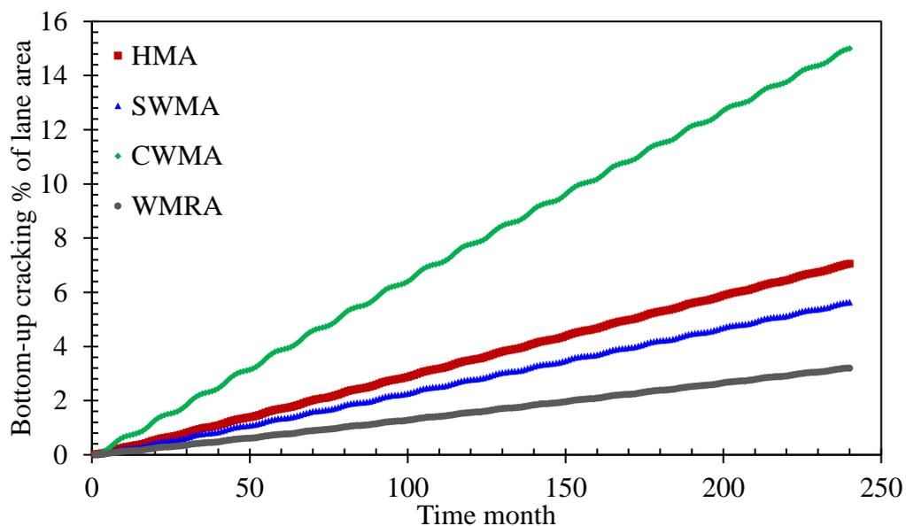
Figure 7-19. Predicted bottom-up fatigue cracking
