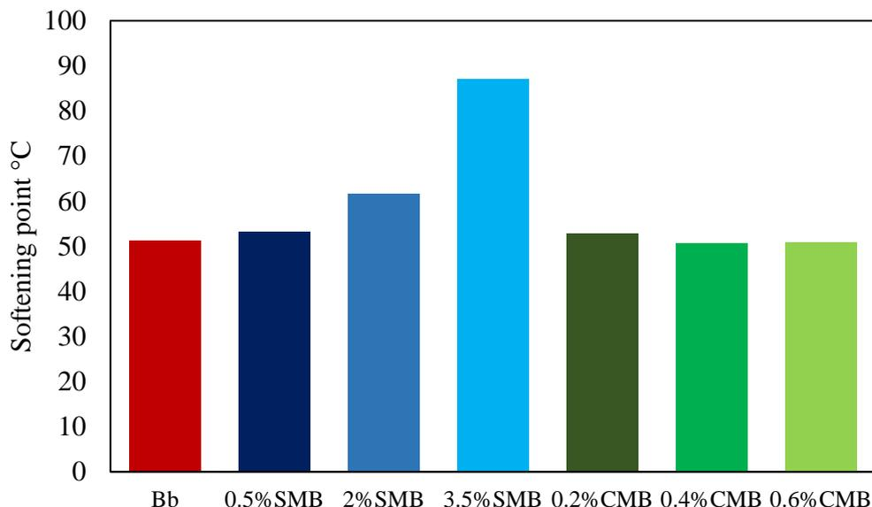
Figure 3-5. Softening point test results
