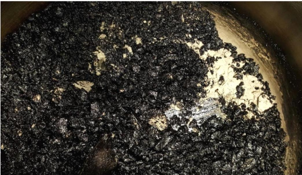
Figure 4-9. Non-standard HMA mixed at 115°C; please note uncoated fines and dust particles when mixing asphalt at 115°C without WMA additives
