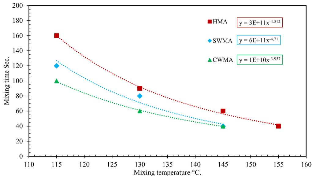
Figure 4-10. Mixing time and temperature relationship
