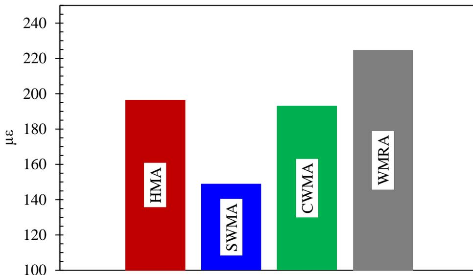
Figure 7-18. Estimated Tensile strain at pavement surface in the hot weather
