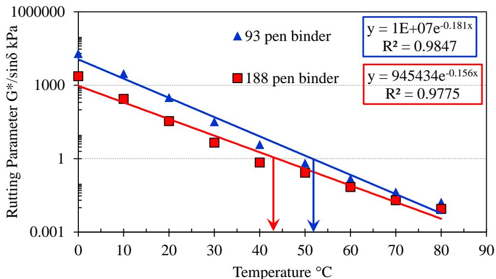
Figure 6-16. Superpave rutting parameters of 188 and 933 dmm pen binders
