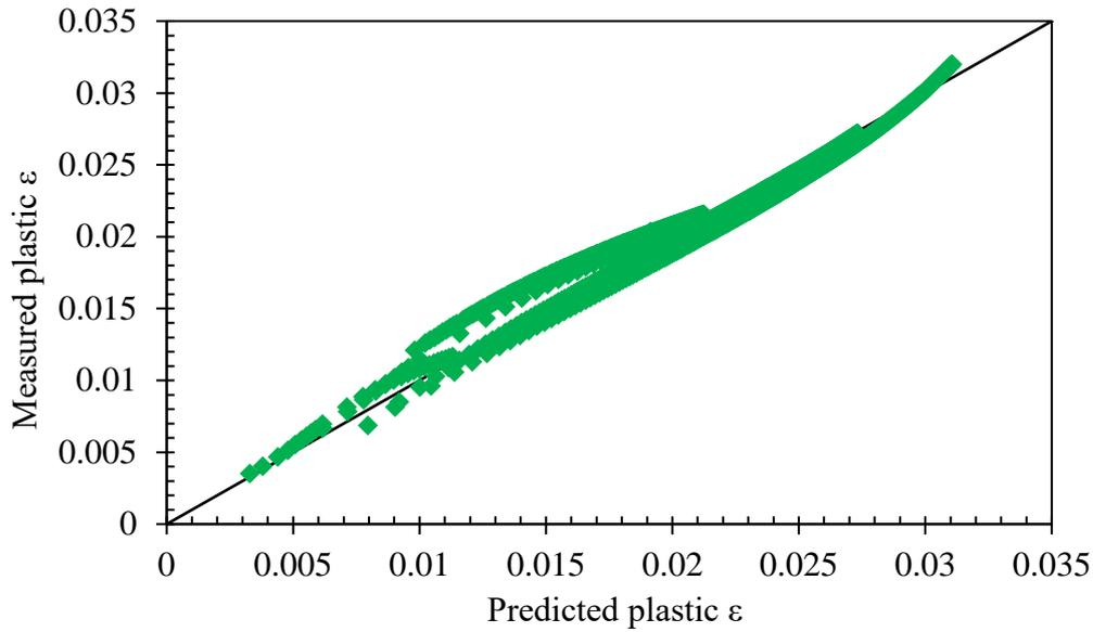
Figure 7-3. Measured and predicted RLAT results of CWMA mix
