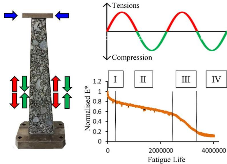
Figure 6-20. Two-point bending typical loading and material response
