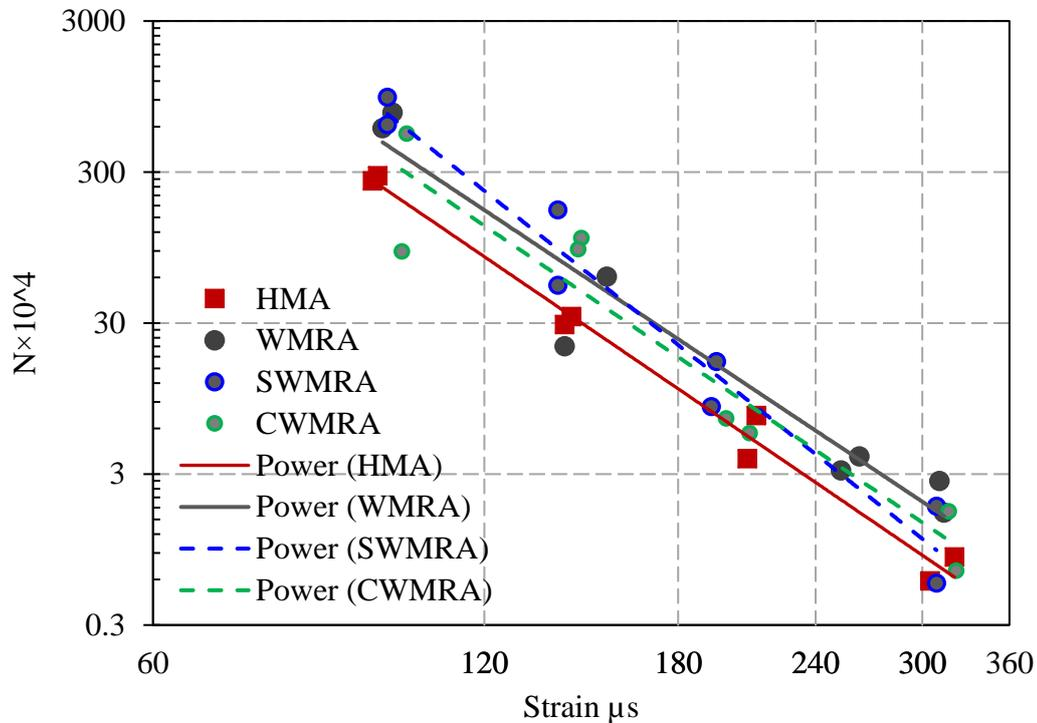
Figure 6-33. Fatigue lines of HMA, WMRA, SWMRA, and CWMRA at 20°C
