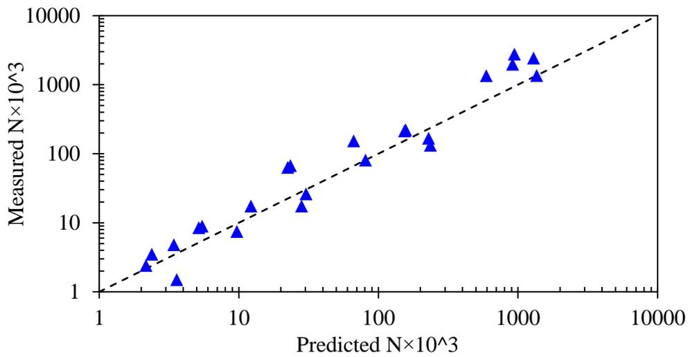
Figure 7-6. Measured versus predicted fatigue life of SWMA
