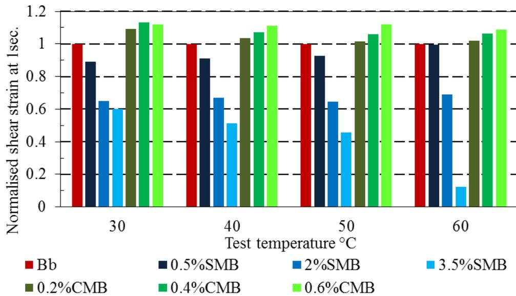
Figure 3-25. Normalised creep results at 1 sec. of loading
