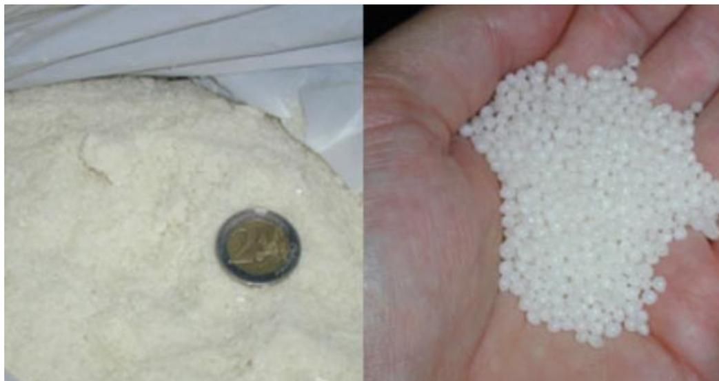
Figure 2-2. Two typical types of Sasobit, flakes to the left and prills to the right. (Hurley and Prowell, 2005)
