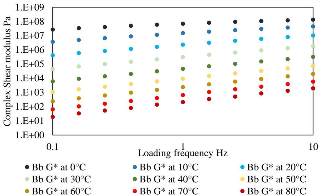
Figure 3-10. Shear modulus results of Bb
