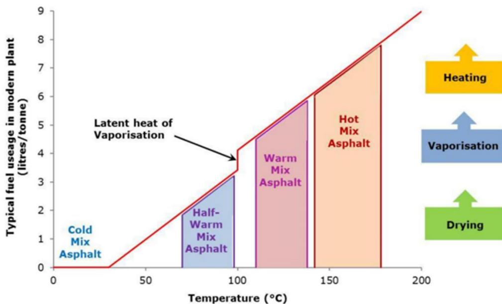
Figure 2-1. Asphalt types based on the mixing temperature
