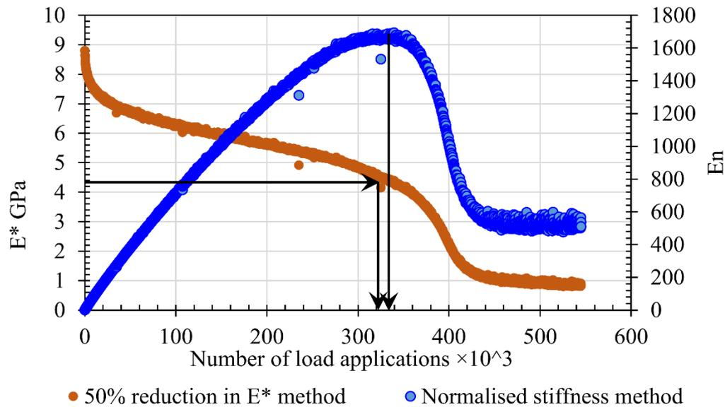
Figure 6-21. Fatigue life determination by modulus reduction and normalisation methods
