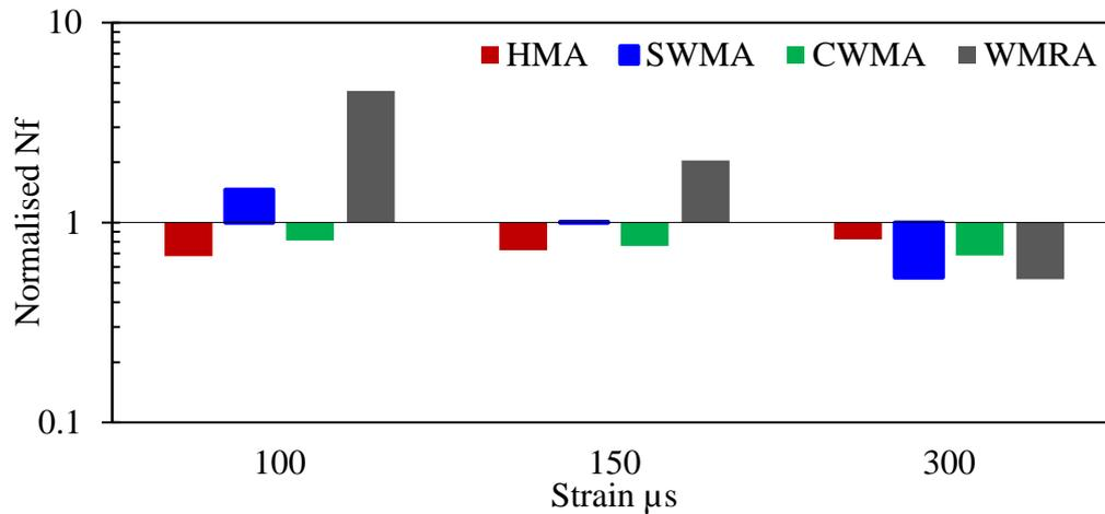
Figure 6-44. Normalised Nf (Nf LTOA / Nf unaged)
