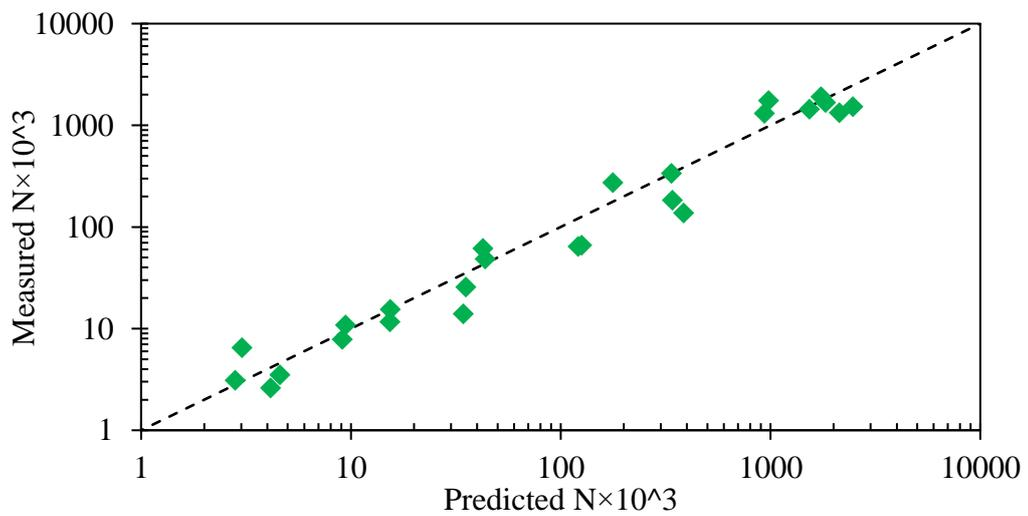
Figure 7-7. Measured versus predicted fatigue life of CWMA
