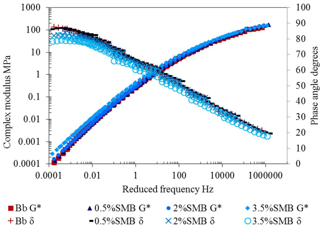
Figure 3-20.  $G^*$  and  $\delta$  results of SMBs after RTFOT+PAV ageing
