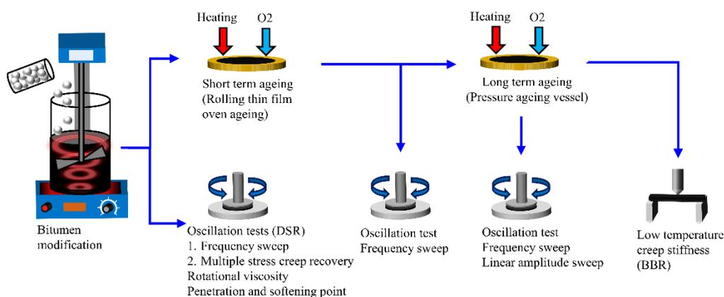
Figure 3-3. Experimental plan of bitumen characterisation
