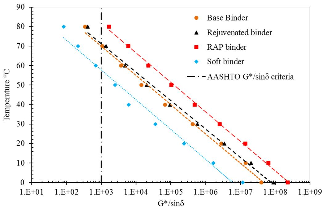
Figure 5-5. Critical high-temperature parameters
