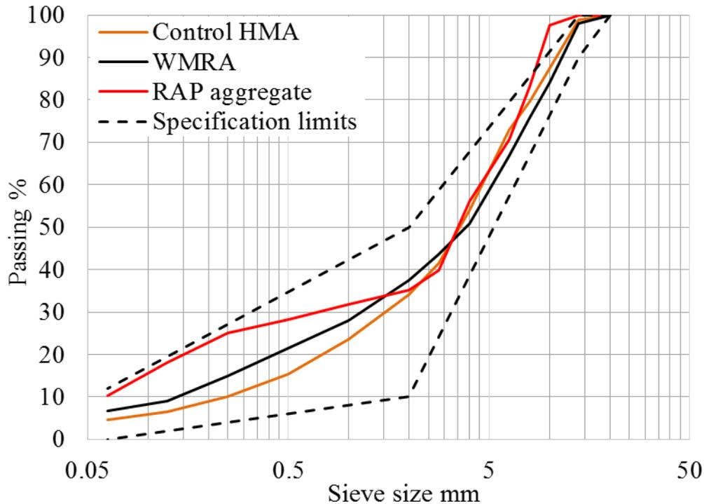
Figure 5-1. Aggregate gradation of the control HMA aggregate, RAP aggregate, and AC mix containing 50% RAP
