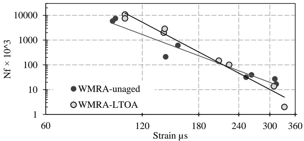
Figure 6-43. Fatigue lines of WMRA before and after ageing
