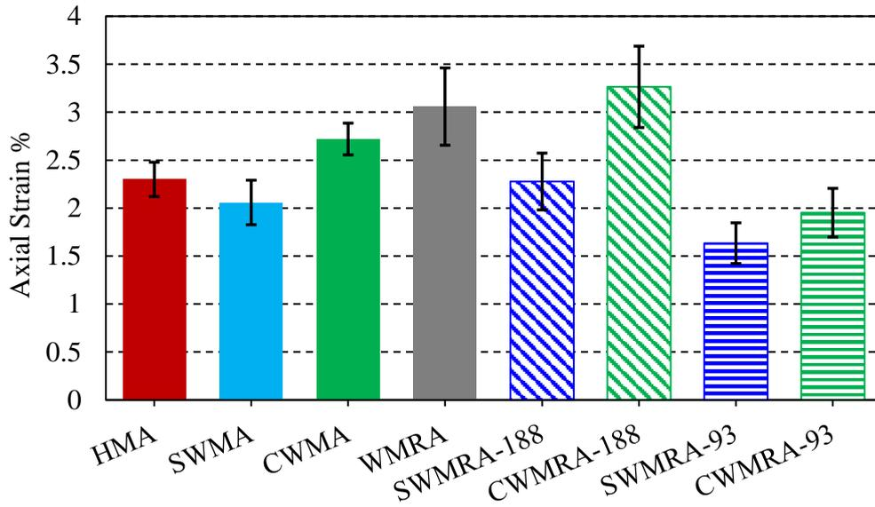
Figure 6-17. RLAT results at 50°C
