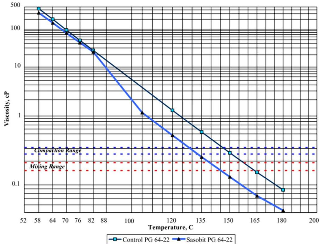
Figure 2-4. Mixing and compaction temperature determination based on binder viscosity (Hurley and Prowell, 2005)
