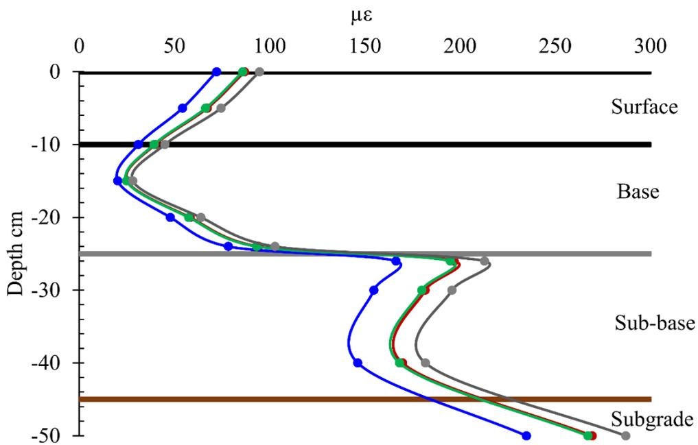
Figure 7-16. Compressive strain levels in the hot weather
