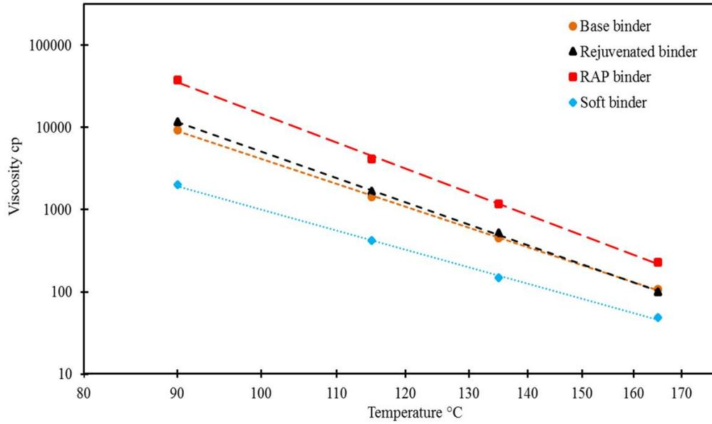
Figure 5-3. Rotational viscosity results
