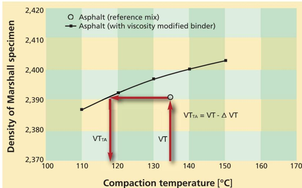
Figure 2-7. Equi-volumetric compaction temperature determination
