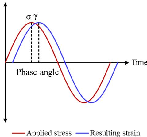
Figure 3-8. Sinusoidal stress-strain relationship
