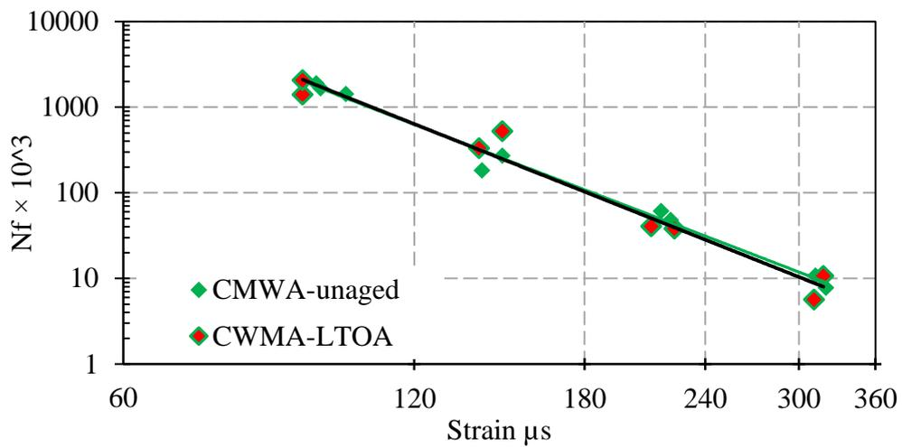
Figure 6-42. Fatigue lines of CWMA before and after ageing
