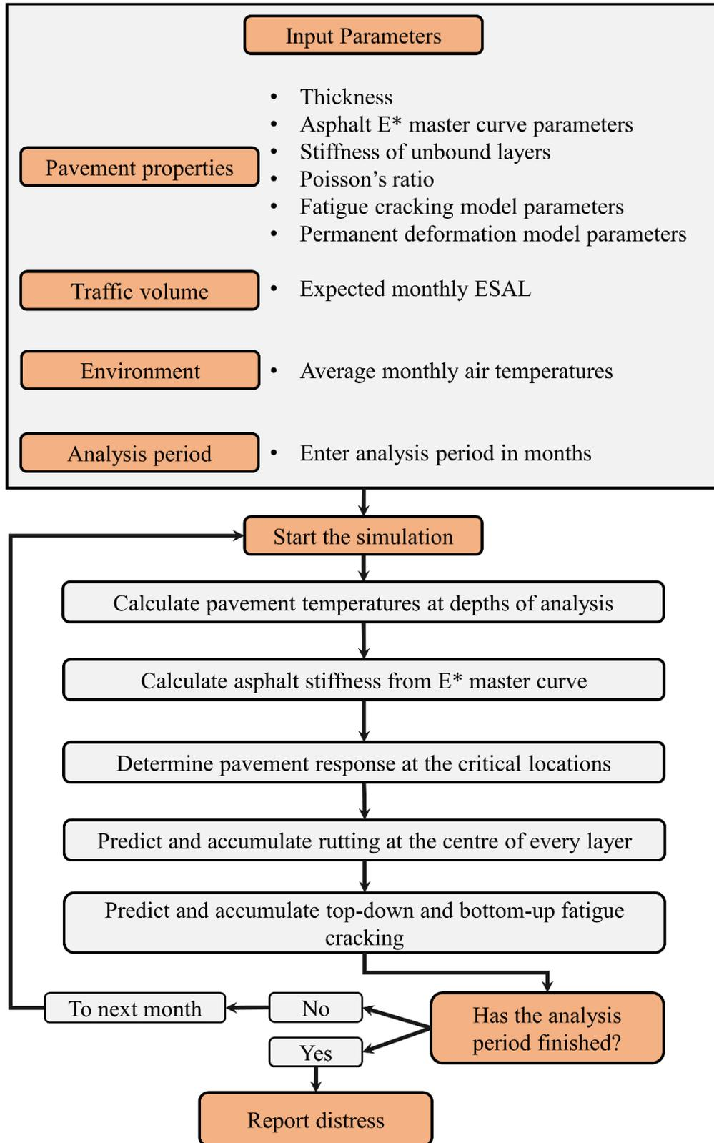
Figure 7-12. A flowchart explaining the method followed to predict pavement performance and its service life
