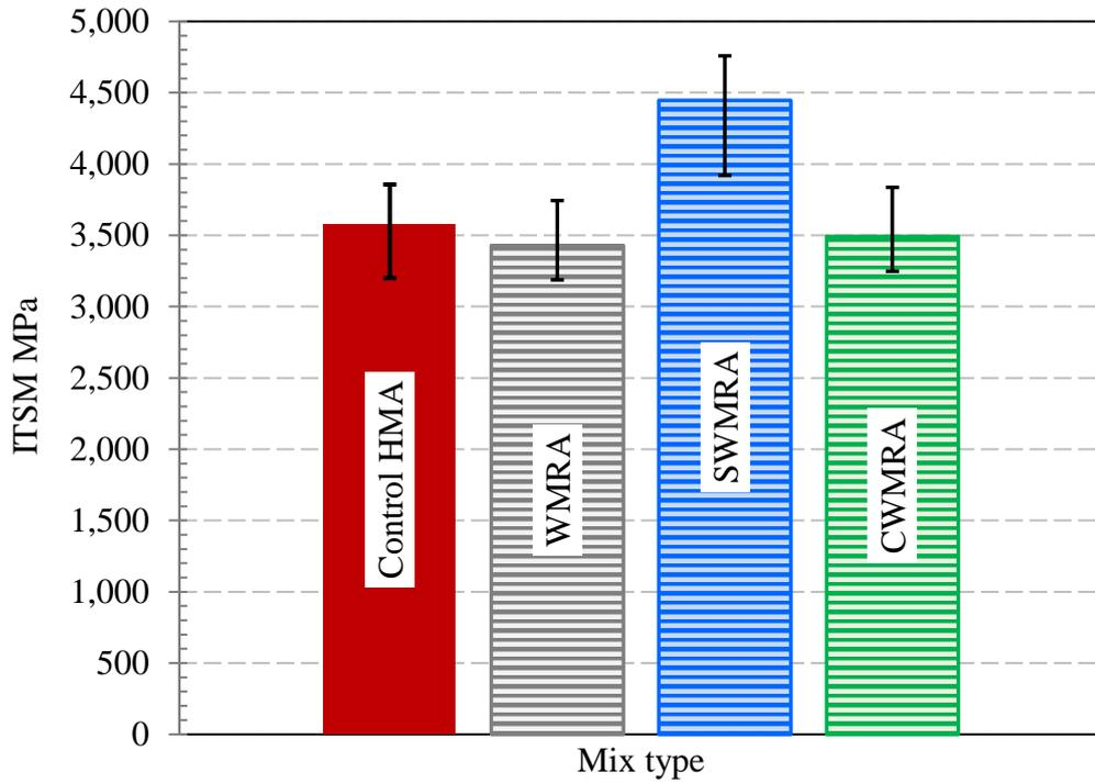
Figure 5-13. ITSM results of 50% RAP mixes produced using WMA additives
