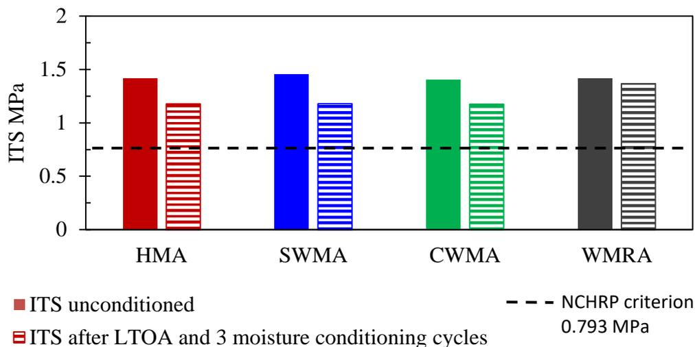
Figure 6-50. ITS measurements after combined LTOA and three MCCs
