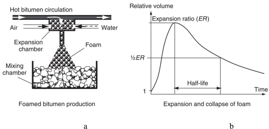
Figure 2-3. Bitumen foaming principles, (a) foaming process, (b) characteristics of foamed bitumen (Thom, 2014)
