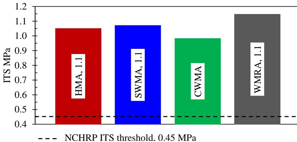
Figure 6-47. ITS results after moisture conditioning
