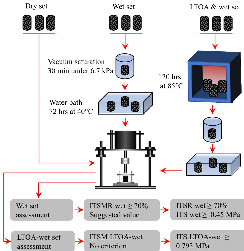
Figure 6-45. Evaluation procedure of MDR
