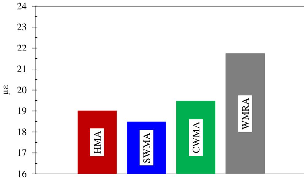
Figure 7-17. Estimated tensile strain at pavement surface in the cold weather
