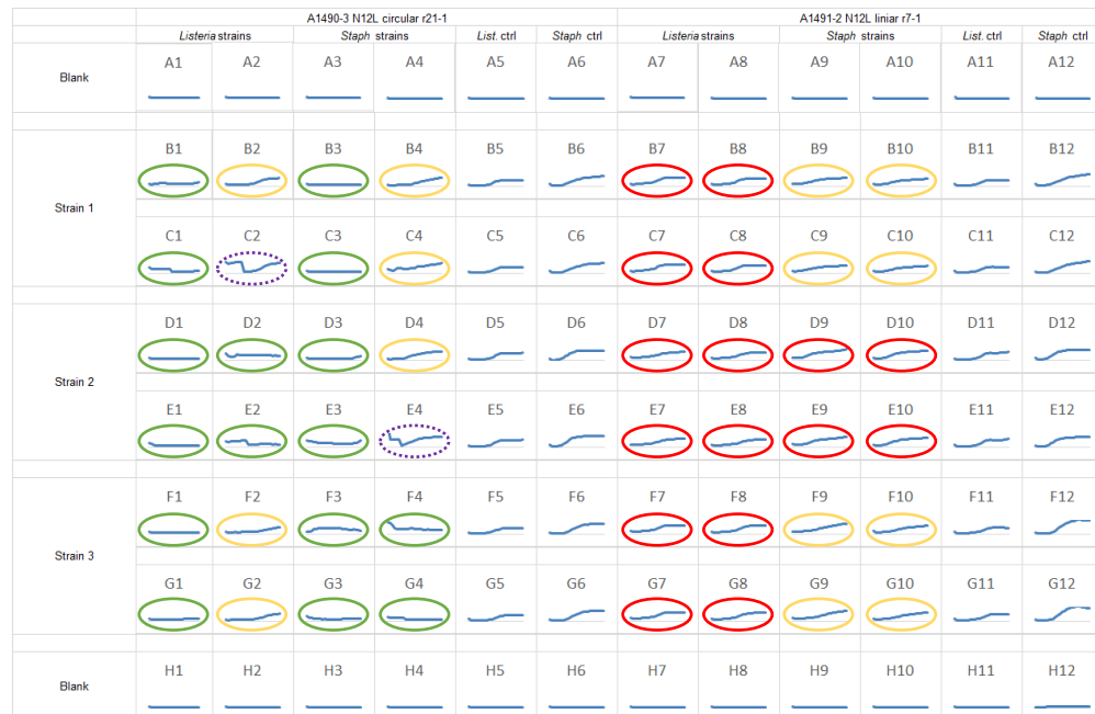
Figure 4.2.1: OD_{620} measured every hour for 24 hours. Microtiter plate layout as shown in table 4.2.1. Green = complete inhibition, yellow = moderate inhibition, red = no inhibition and dashed purple = inconclusive.
