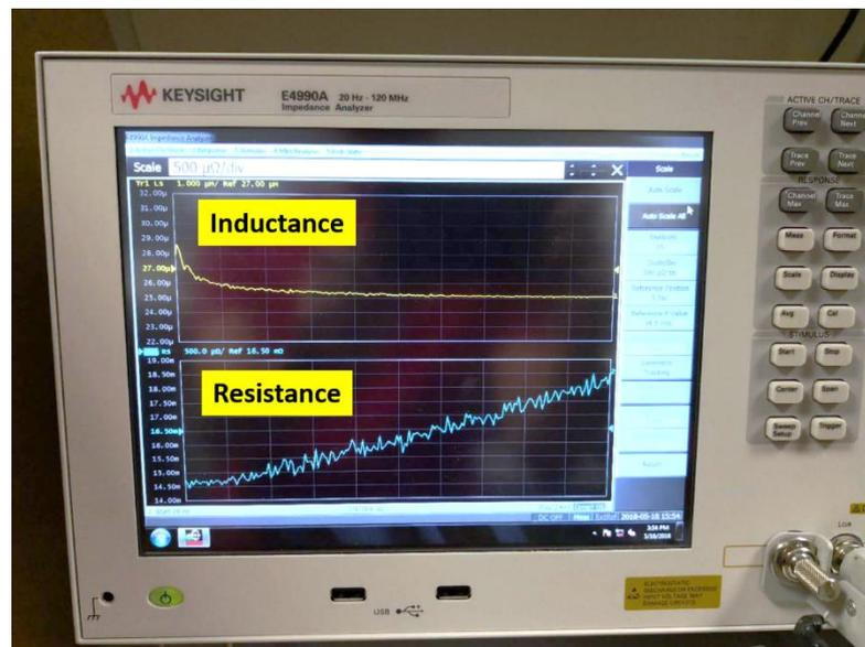
(b) Frequency response of inductance and resistance of winding in the motorette
