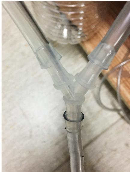
*Figure 3.15 – Y-shaped connector used.*
