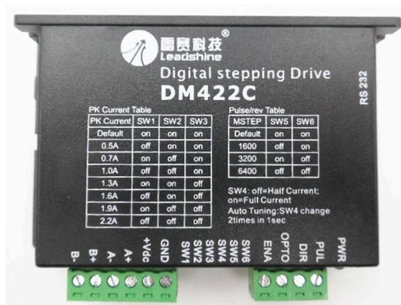
Figure 3.12 – Image of DM422C stepper driver used.
