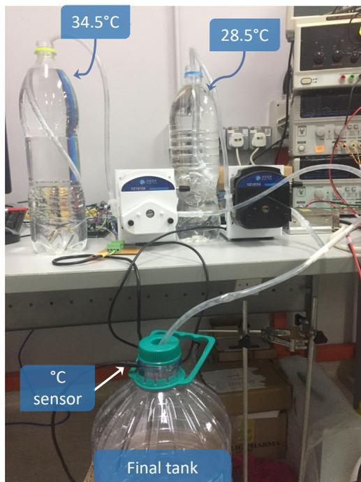
Figure 5.2 – Experimental setup for a simplified temperature controller.
