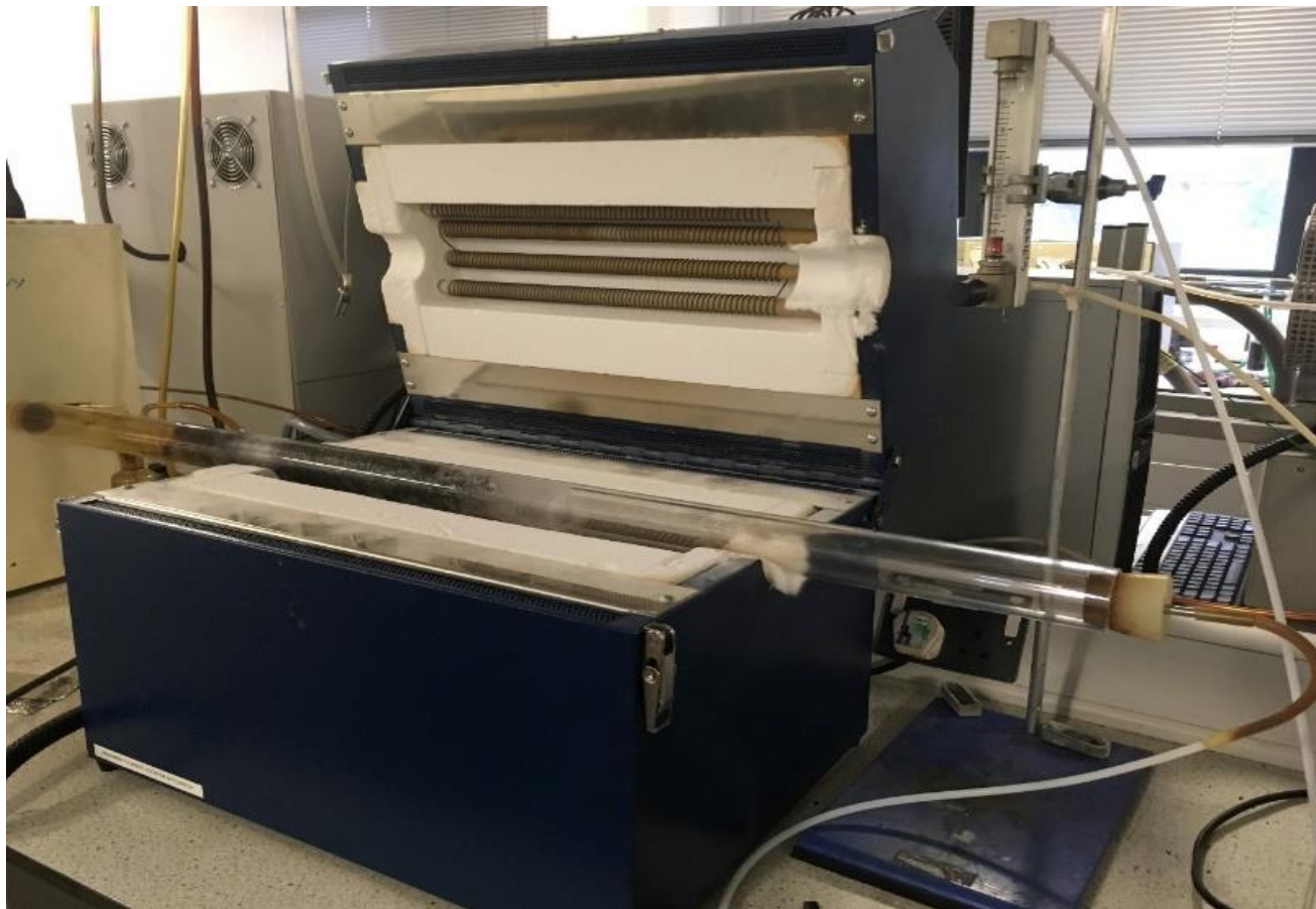
Figure 3.3 Horizontal tube furnace used in torrefaction experiments
