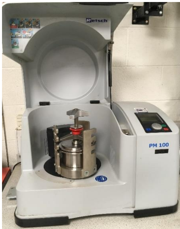
Figure 3.4 Ground bagasse in ball mill (top) and fully assembled ball mill (bottom)
