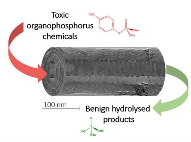
Figure 3.4. Schematic diagram utilising carbon nanoreactors to promote hydrolysis of OP agents to facilitate decontamination.
