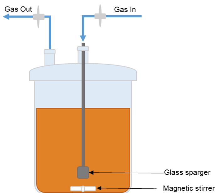
Figure 2.1 Oxygenation procedure used for wort preparation.
