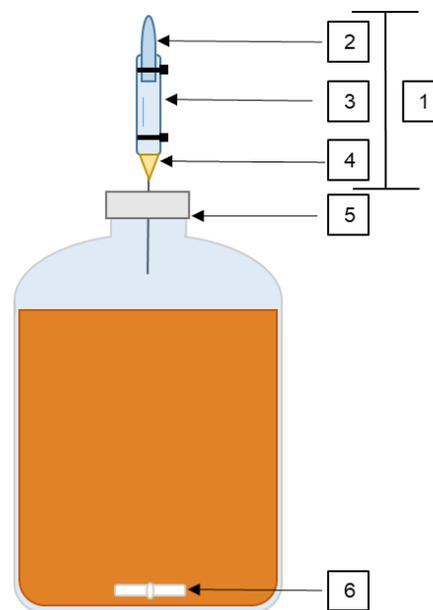
Figure 2.2 Mini fermentation vessel design (100mL working volume). 1: Bunsen valve; 2: Glass Durham tube; 3: Silicon tubing with opening; 4: Needle; 5: Metallic crimp covering rubber septum; 6: Magnetic stirrer.
