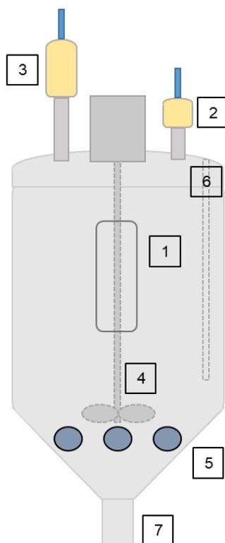
Figure 2.3 Infors fermenter configuration. 1: Viewing port; 2: Gas inflow passed through a HEPA filter; 3: Gas outlet, first through a condenser then a HEPA filter; 4: Impeller to achieve required mixing; 5: Ports for pH probe, and DO probe; 6: Temperature probe; 7: Sampling port, which can be steam sterilised or flushed with ethanol.
