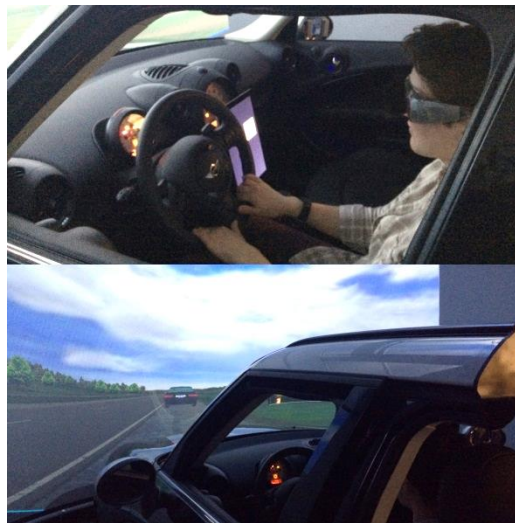
Figure 17. Medium-fidelity driving simulator at Virginia Tech
