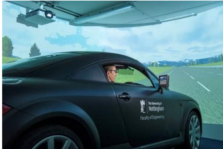
Figure 16. Driving simulator at the University of Nottingham Human Factors Research Group (Audi TT)
