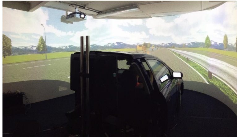
Figure 15. Driving simulator at the University of Nottingham Human Factors Research Group (Honda)
