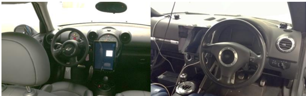
Figure 19. Location of the in-vehicle touch screens in the user trials (Left: Virginia Tech driving simulator, Right: University of Nottingham driving simulator)
