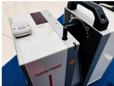
Fig.4.15 UWB transmitter mounted on the top of HDS7000 scanner
