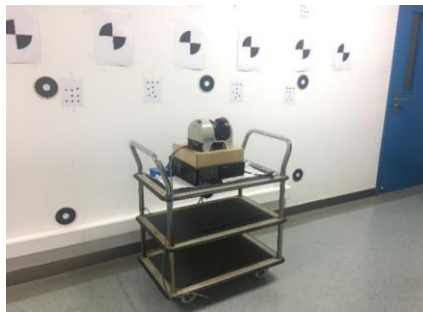
Fig.4.8 Laser scanner and IMU mounted on a trolley
