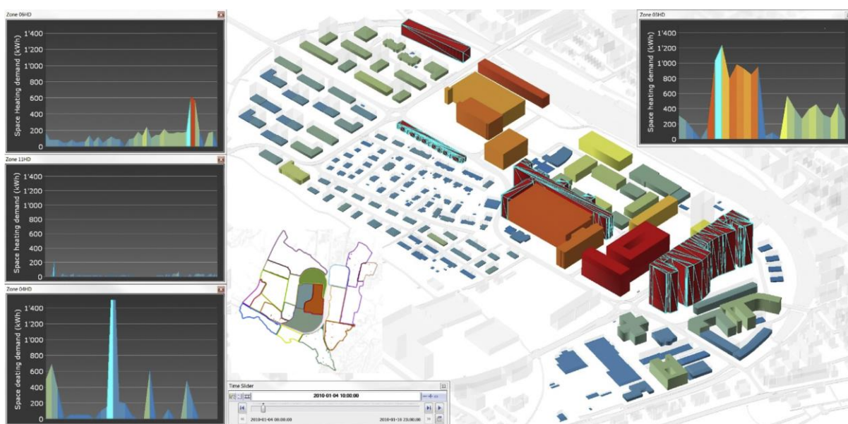
Fig. 2-11: Spatio-temporal energy map of space heating demand of a city district in Switzerland [2.53]
