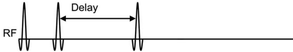
Figure 45: Schematic representation of the SPAMM sequence consisting of a prepulse. Diagram authored by Sprengers et al 218 .
