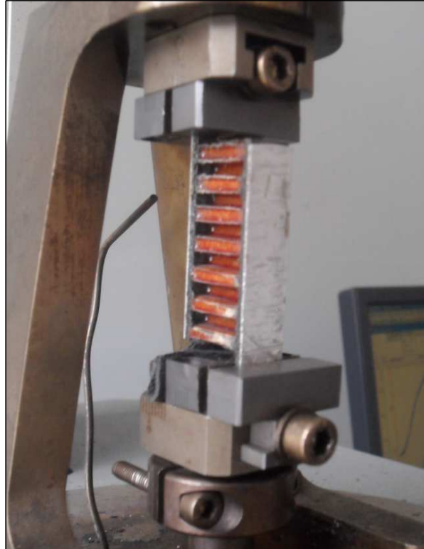
Figure 3.3: Configuration of the segment of the core under shear deformation in the TMA device
