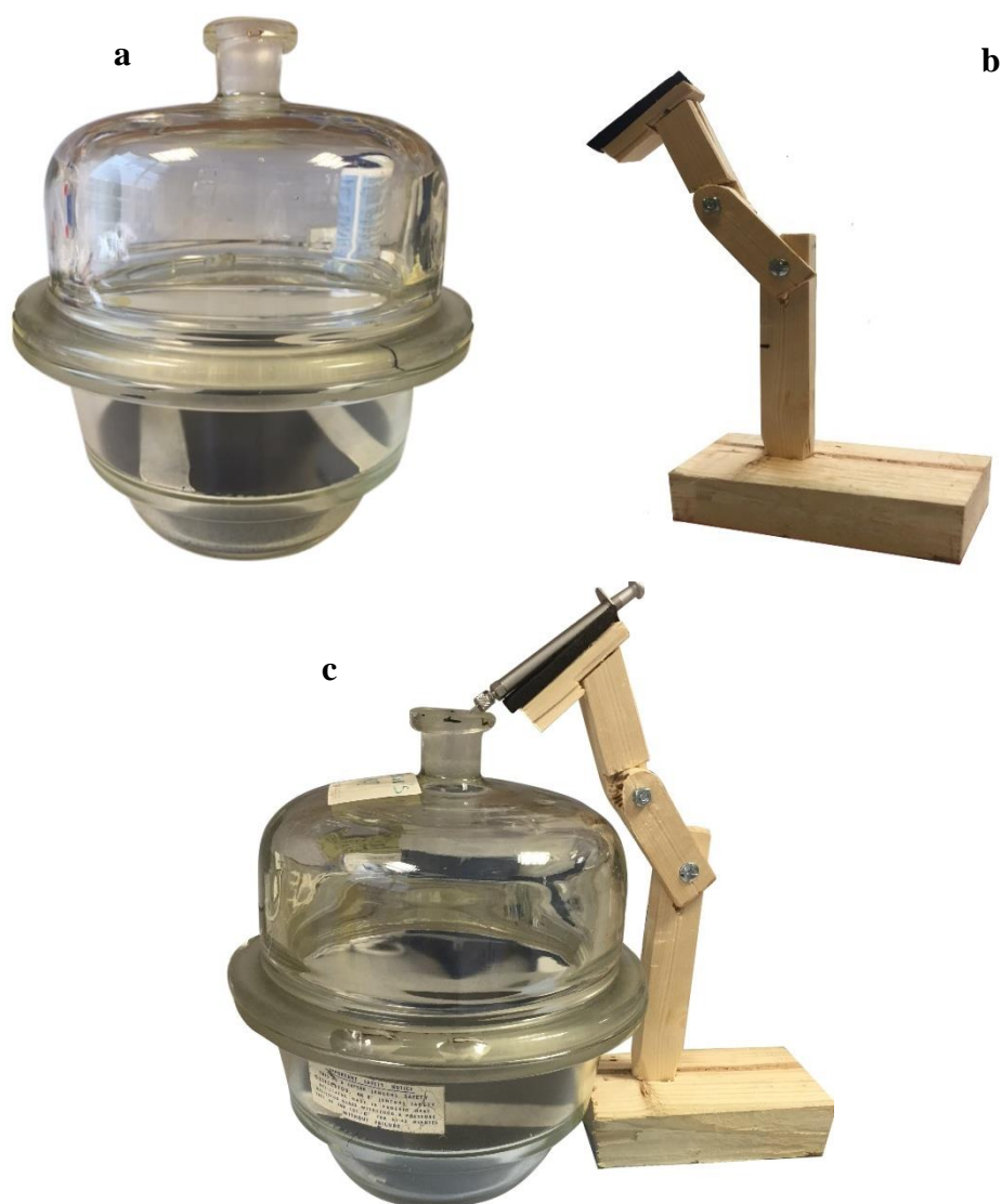
Figure 4.2.2. The deposition system. (a) The vacuum glass desiccator. (b) The stand which ensures the consistency of the spraying point (c) The final deposition system, assembled as a Penn-Century MicroSprayer® Aerosoliser (IA-1C) connected to the high-pressure syringe (FMJ-250) and held in position by the stand. Sample solutions are sprayed inside the holder glass desiccator system.
