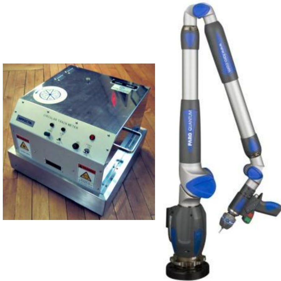
Figure 2.21: Circular Texture Meter (left) and FaroArm-Platinum (right) (Applied Pavement Technology, 2008; Faro, 2014)
