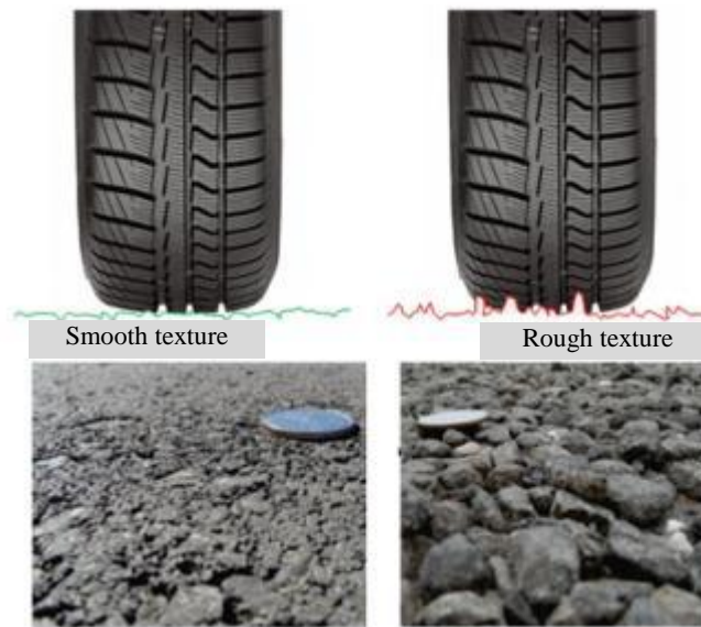
Figure 2.12: Tyre/Pavement contact area in rough and smooth texture (Nutz and Hoffmann, 2012)
