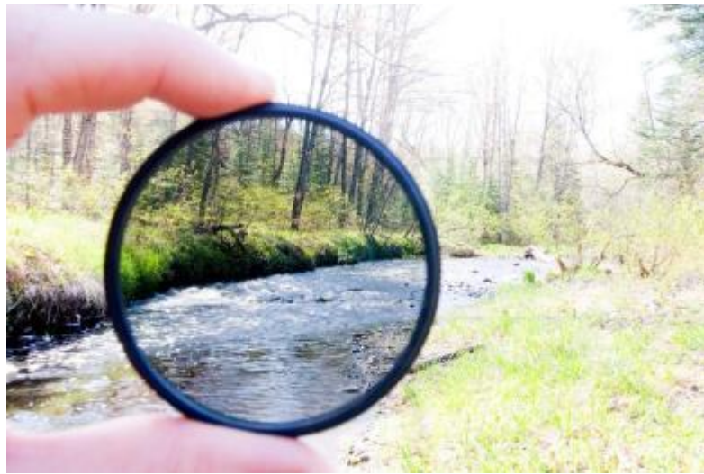
Figure 2.15: Demonstration of the effect of the neutral density filter (Wiki, 2014)
