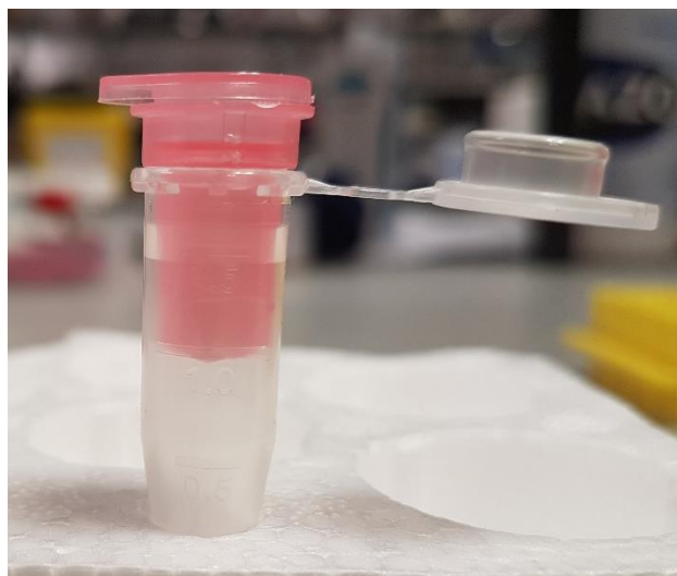
Figure 4.16: The dialysis device employed for the release study. The IDR 1018-sodium usnate complex-loaded-nanoparticles suspension is added to the device, which can be easily fitted into a 2 mL eppendorf. The two released components of the complex, IDR 1018 and sodium usnate, migrate from the dialysis device to the eppendorf through the dialysis membrane located at the bottom of the device.
