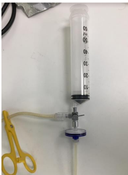
Figure 7 – Methane gas inlet pipe attached to syringe and 0.22 \mu\text{m} filter used for dispensing methane gas into cultures.
