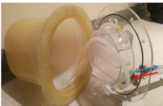
Figure 4.1: A sample holder into which water was directly pumped for temperature-controlled imaging, was built to fit inside the RF head coil.
