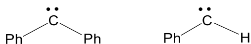
Figure 17. Examples of carbenes with calculated angles and separation energy for the singlet and triplet states. Left ( 2.94 \text{ kcal mol}^{-1} , 119.5^\circ for singlet state, 142.88^\circ for the triplet state), Right ( 2.75 \text{ kcal mol}^{-1} , 106.96^\circ for singlet state, 135.67^\circ for the triplet state). 70
