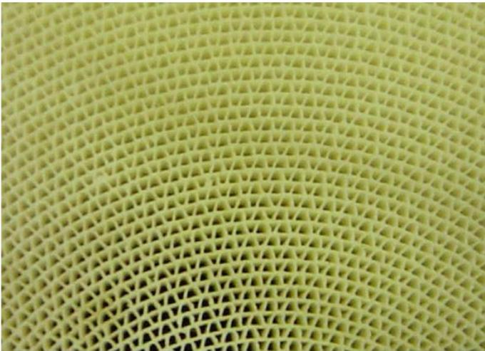
Fig 2-6 Honeycomb air channels of desiccant wheel [28]
