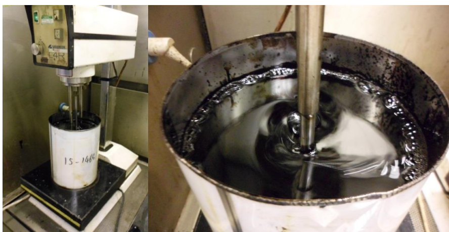
Figure 29: Bulk ageing procedure using HSM
