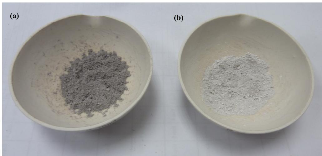
Figure 3.2: Different wt% of ZnO/Fe<sub>3</sub>O<sub>4</sub> powders after mechanical mixing. (a) 20 wt% of Fe<sub>3</sub>O<sub>4</sub>; (b) 1 wt% of Fe<sub>3</sub>O<sub>4</sub>.
