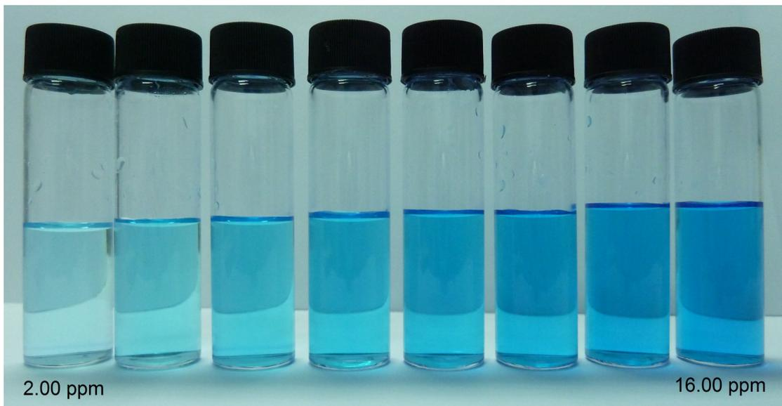
Figure 3.12 Eight different concentration of the MB dye solutions in vials.
