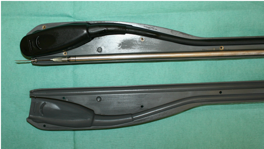
Figure 3.3. An early model transvaginal casing opened to show the positioning of the ultrasound transducer and needle guide.
