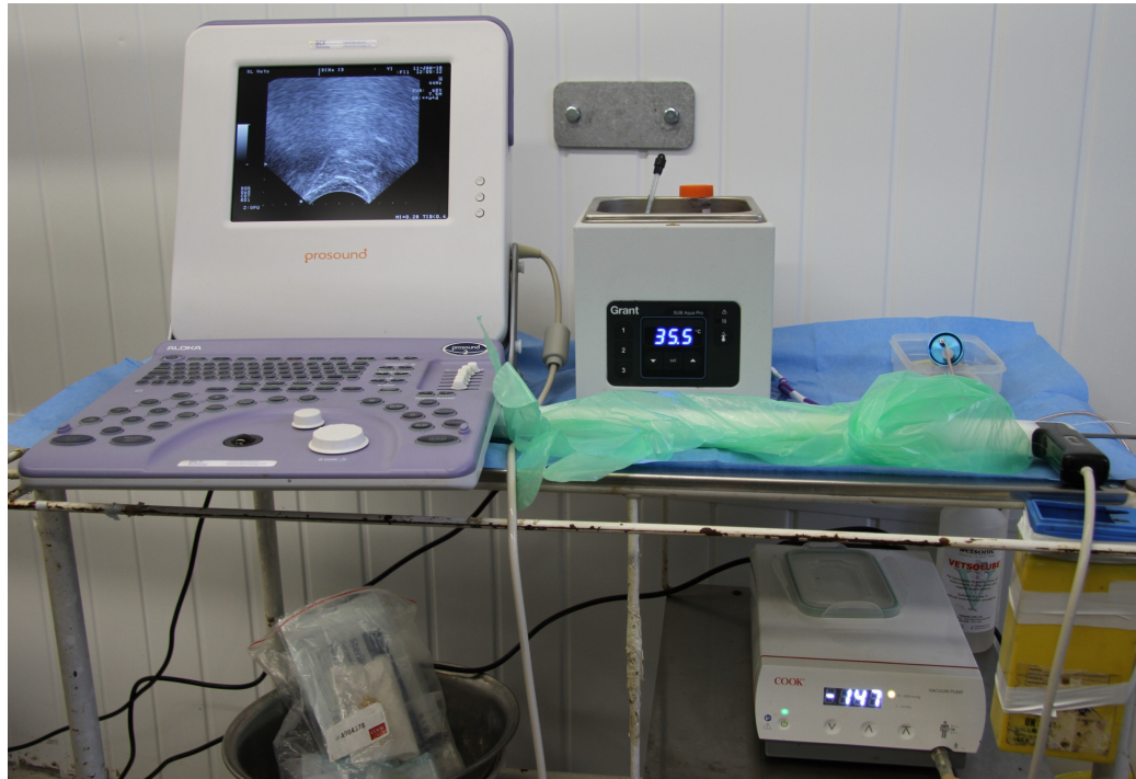
Figure 3.7. A Prosound 2® ultrasound machine showing handle prepared for transvaginal insertion, stainless steel needle guide, water bath and vacuum pump (below).
