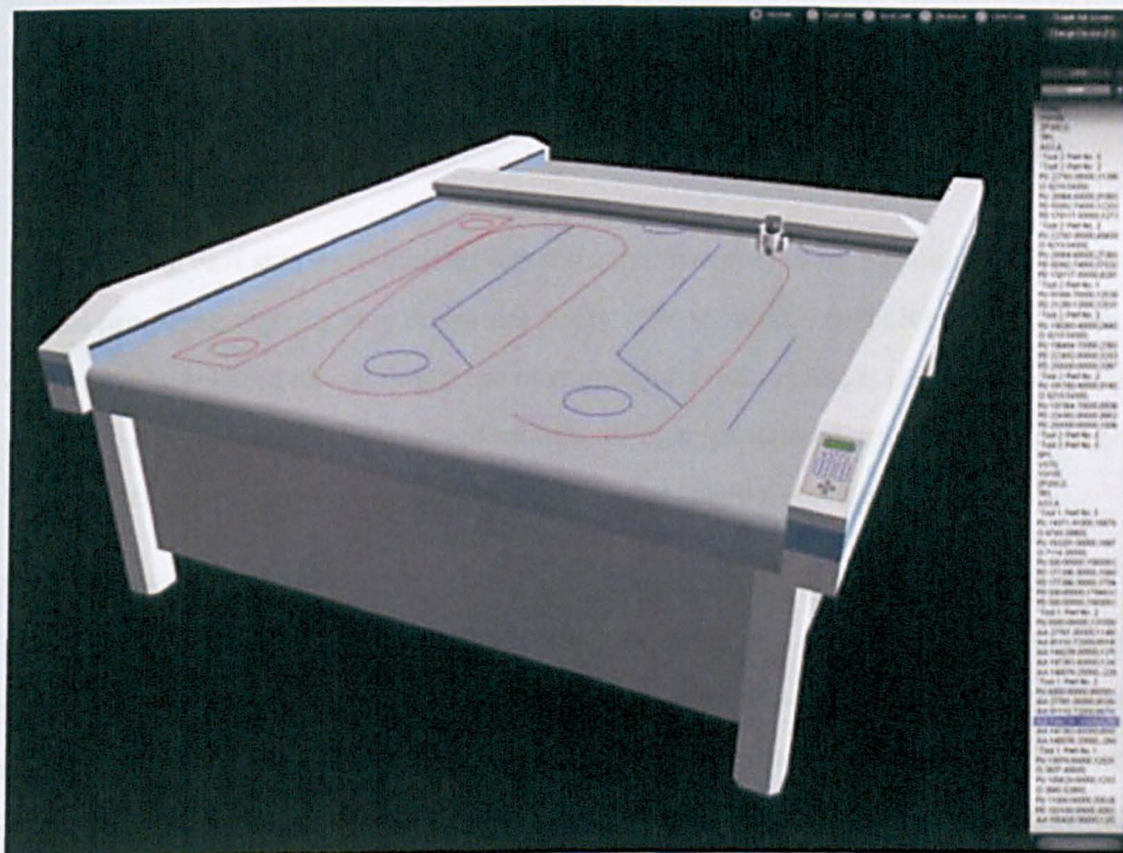
Figure 92. VMach application simulating a Zund Machine cutting HPGL instructions
