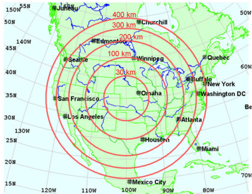
Figure 1-9 Diagram depicting the potential areas affected by HEMP in relation to the height of burst [17].
