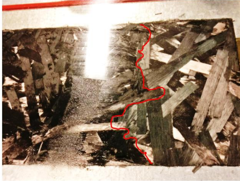
Figure 5.7 Typical profile of flow front from a DCFP preform during an in-plane permeability test
