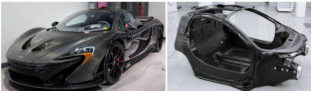
Figure 1.1 McLaren P1 MSO carbon series and its carbon tub
