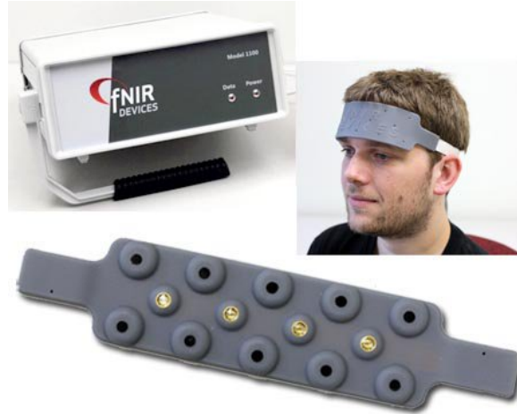
Fig. 4.4 The fNIRS 300 sensor [69]
