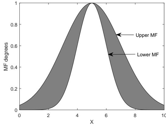
Figure 2.3: A Gaussian interval type-2 membership function
