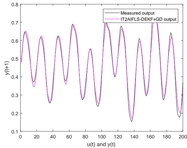
Figure 6.5: Actual and predicted output using hybrid IT2AIFLS for second-order system identification problem #1
