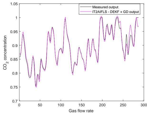
Figure 6.9: Actual and predicted output of gas furnace time series using IT2AIFLS trained with DEKF+GD
