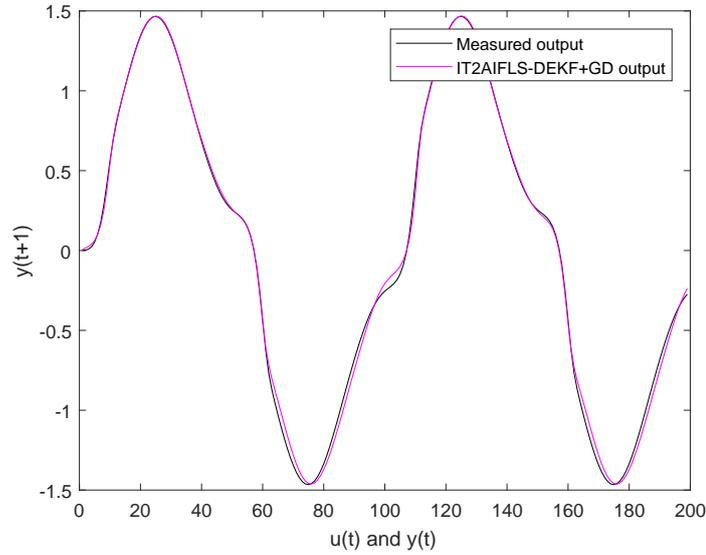
Figure 6.6: Actual and predicted values for system identification#2 using IT2AIFLS
