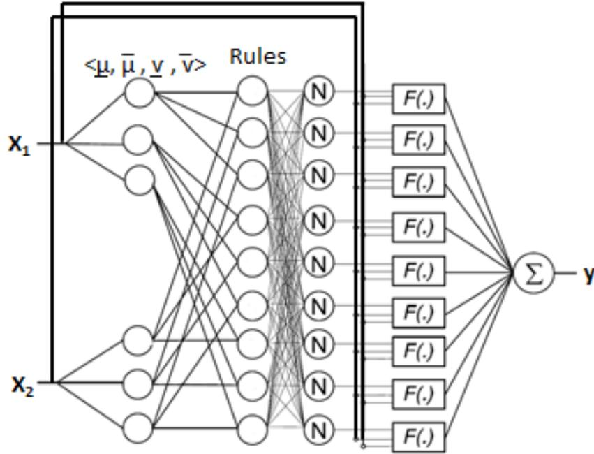
Figure 3.5: An IT2AIFLS Structure - adapted from [4]
