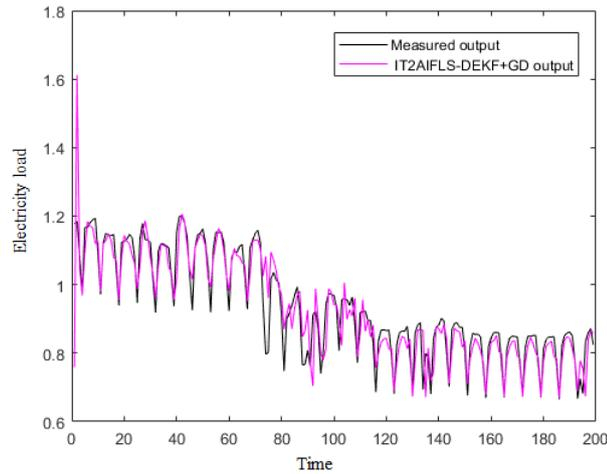
Figure 6.8: Actual and predicted values of Poland electricity load with IT2AIFLS on test dataset
