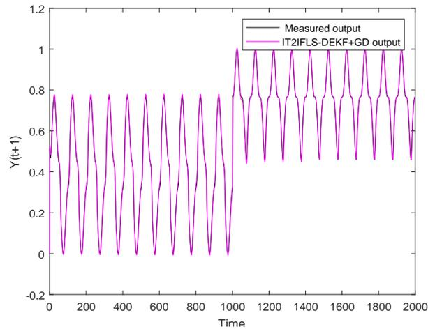
Figure 5.1: Actual and predicted output using IT2AIFLS for identification problem
