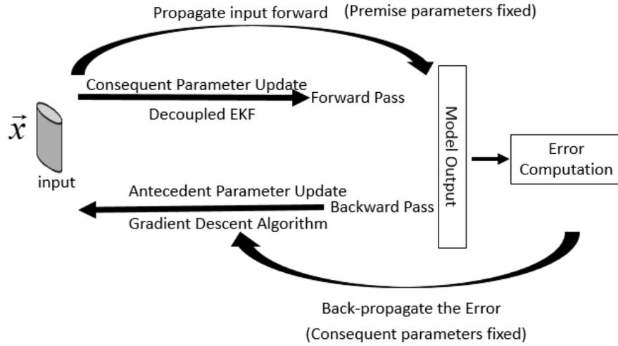
Figure 6.1: Hybrid learning procedure of IT2AIFLS using DEKF and GD
