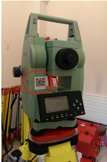
Figure 4.4: Theodolite with QR-code
