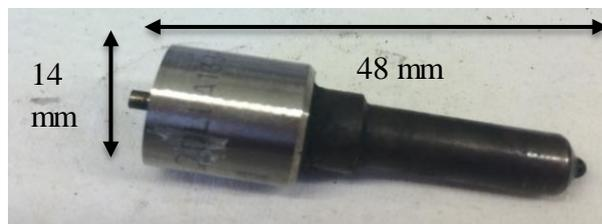
*Figure 2.2 Photo of an injector tip.*
