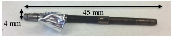
*Figure 2.3 Photo of a push rod.*
