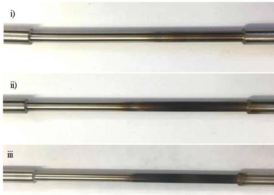
*Figure 6.2 Visual photos of JFTOT tube 1-3. i) JFTOT 1 was fuelled on B20 RME biodiesel fuel at 260 °C for 150 mins. ii) JFTOT 2 was fuelled on ULSD fuel at 260 °C for 150 mins. iii) JFTOT 3 was fuelled on B20 RME biodiesel and ULSD fuel at 260 °C for 450 mins.*
