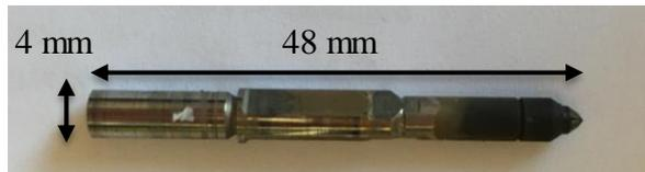
*Figure 2.1 Photo of an injector needle.*
