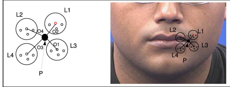
FIGURE 3.26: The configuration of a rigid flock of linear predictors in (Ong & Bowden, 2011). The position of the flock is defined by reference point P and the flock consists of separate linear predictors, denoted as (L1, L2, L3, L4) . Each of the linear predictor has a rigid offset from point P , which are O1, O2, O3, O4 separately.
