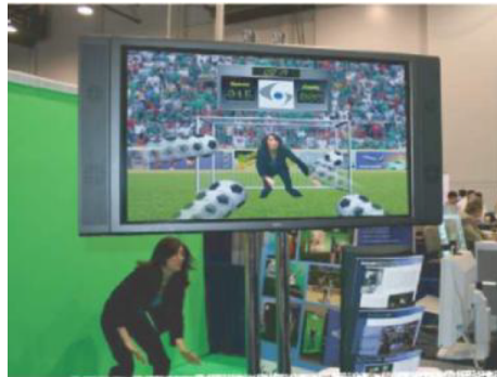
FIGURE 1.4: The example of visual tracking in an interactive game. The camera uses tracking technology to capture the gestures that are converted into gaming actions. This figure is from (Maggio & Cavallaro, 2011).
