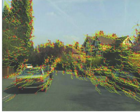
FIGURE 1.1: An example of a camera tracker that uses the information obtained by tracking image patches. The figure is from (Maggio & Cavallaro, 2011).
