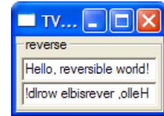
Figure 3.3: A Tangible Value and the GUI generated for it based on the (function) type of the CTV , with text boxes being used to interact with Strings .
