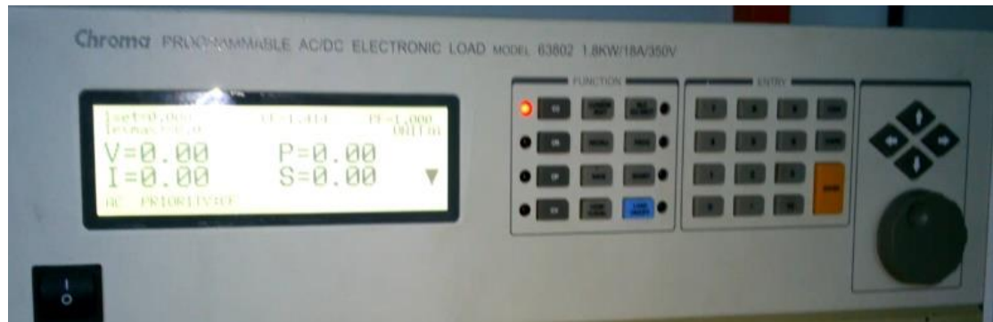
Figure 13. Chroma's 63800 Series AC&DC Electronic Loads
