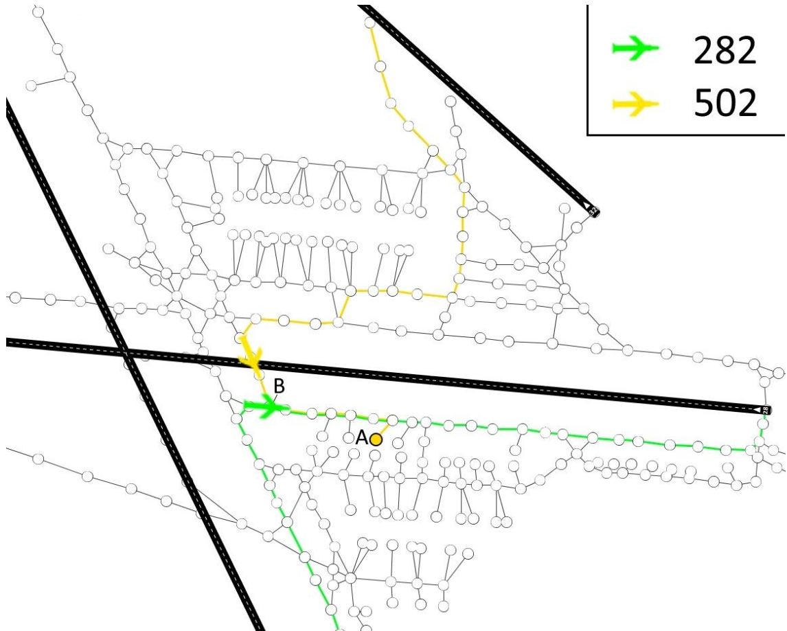
Figure 6.12: An example in Zurich airport where removing taxiways introduces a delay
