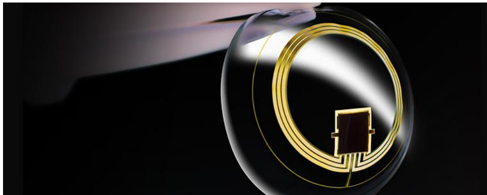
FIGURE 27: (REPRODUCED) SENSIMED TRIGGERFISH® CONTACT LENS SENSOR (SENSIMED, 2014).
